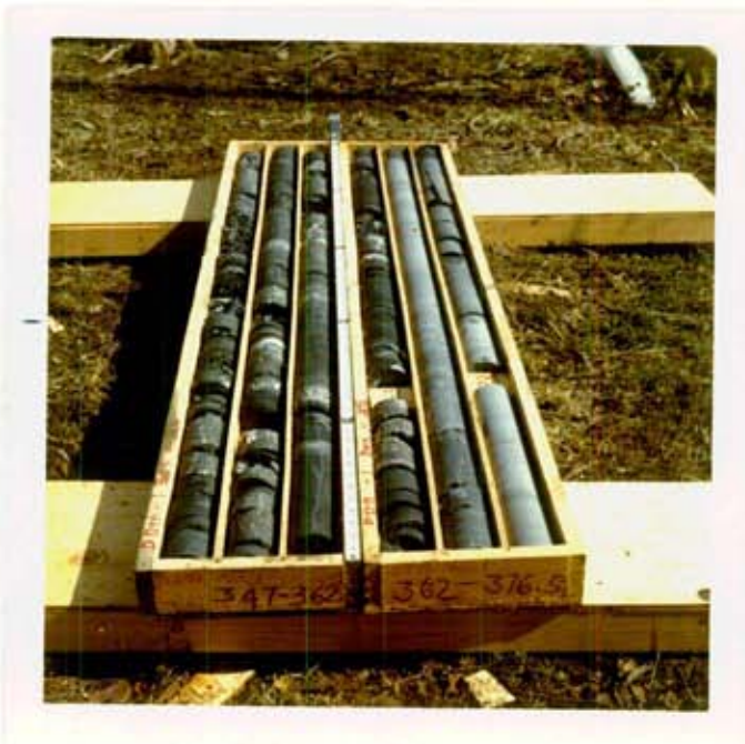
Figure 27.- Part of core with a coal seam from diamond drill hole number one.
