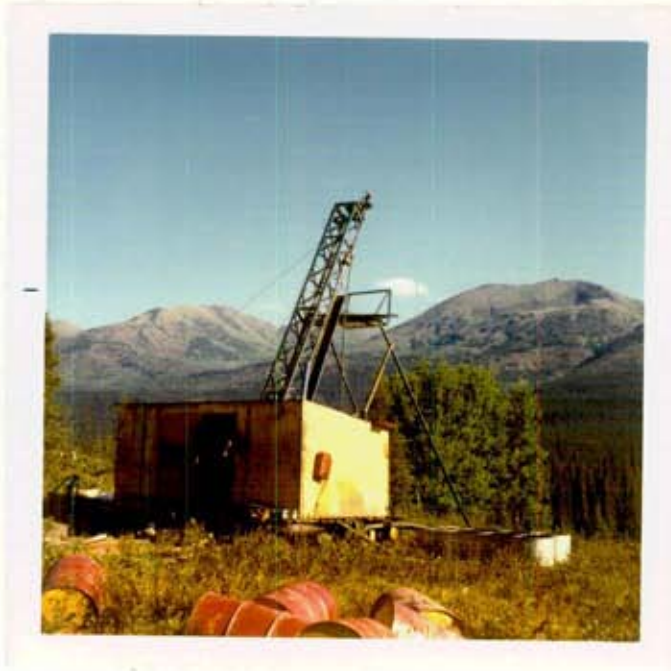
Figure 26.- Diamond drill at drill hole number one. Drilling minus 60 degrees to the southwest. Mount Alec in right background.
