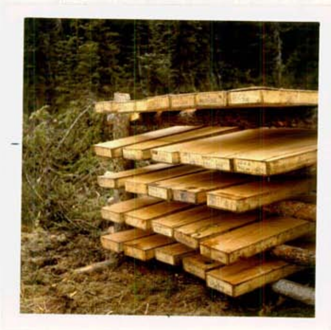
Figure 31.- Core storage at diamond drill hole number six. Core was stored in covered boxes at the site of each drill hole.
