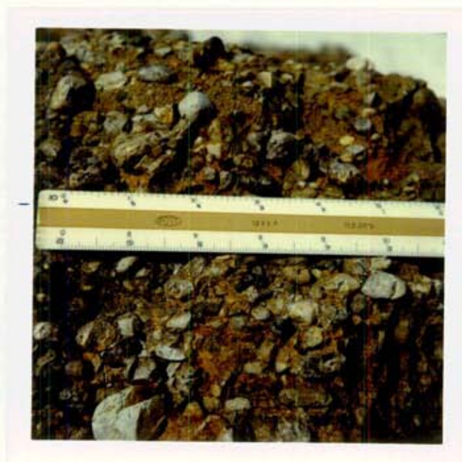
Figure 13.- Photograph of typical specimen of Devil's Claw conglomerate. Pebbles are mostly chert.
