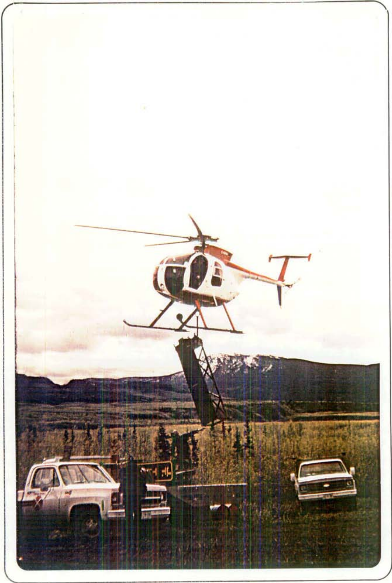
FIGURE 4 - DRILL MOVE USING THE HUGHES 500D HELICOPTER
