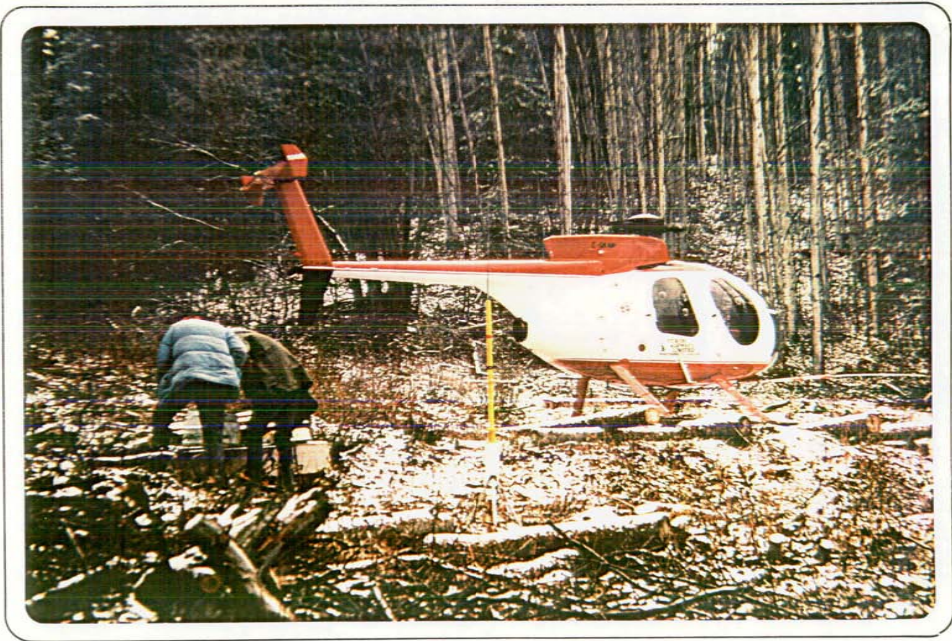
FIGURE 3 - SURVEYING DRILLSITE TDD 79-02 USING THE MARINAV CORP. SATELLITE SURVEY INSTRUMENT
