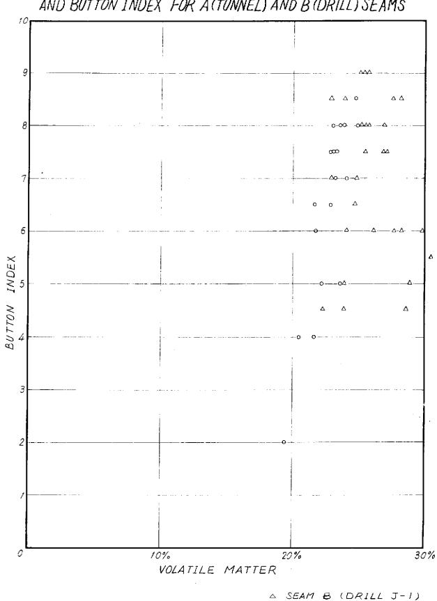
DIAGAM SHOWING RELATION BETWEEN VOLATILE MATTER AND BUTTON INDEX FOR A (TUNNEL) AND B (DRILL) SEAMS
