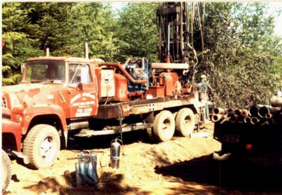
PLATE I. - Bucyrus Erie Model 24R drilling rig used in Hamilton Lake drilling and coring operations.
