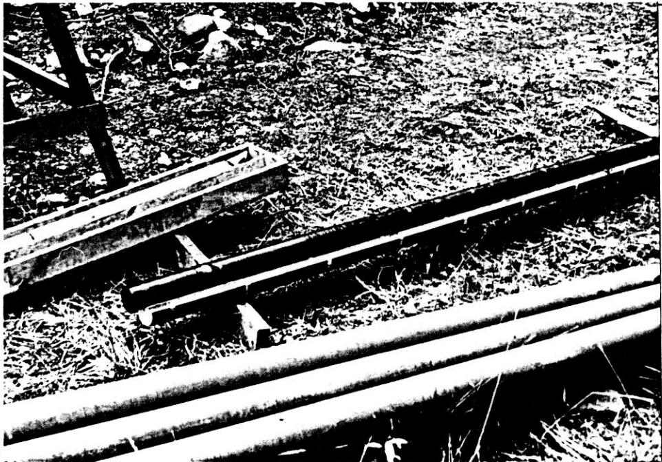
PLATES V and VI: Inner Barrel Removed from Assembly and Split Open for Removal of No. 2 Seam Core.
