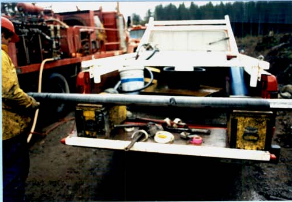
TEN FOOT CORE OF SANDSTONE IN THE SPLIT TUBE CORE BARREL AT DRILL HOLE 88-05
