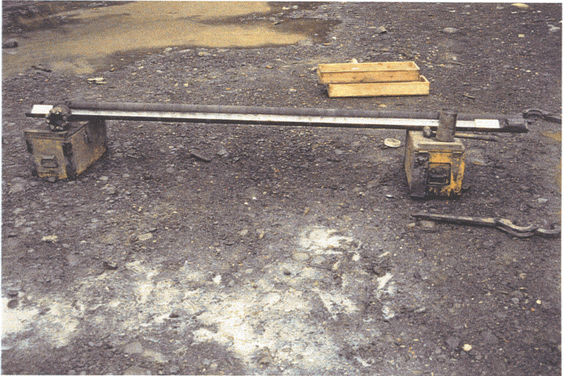
Entire 10 foot Core Run In Split Tube Core Barrel
