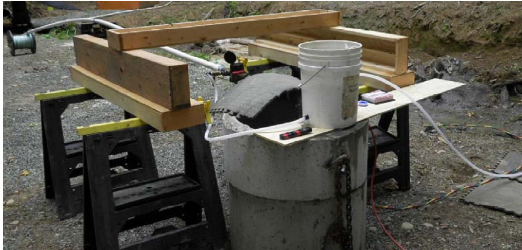
Plate 1: Flow meter camera and discharge water monitoring apparatus (arrow indicates Location water samples were collected from discharge water quality monitoring tube)
