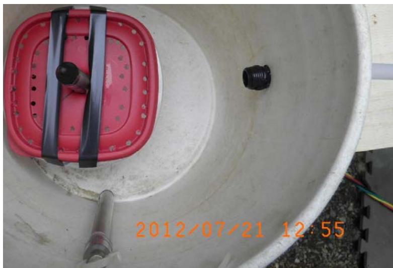
Plate 3: Flow through cell in 20 L PVC pail showing Aqua Troll 200 LTC sensor and discharge point
