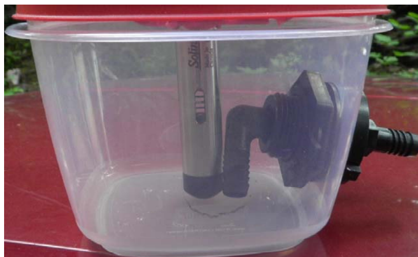
Plate 2: Flow through cell for measuring pump discharge water conductivity and temperature
