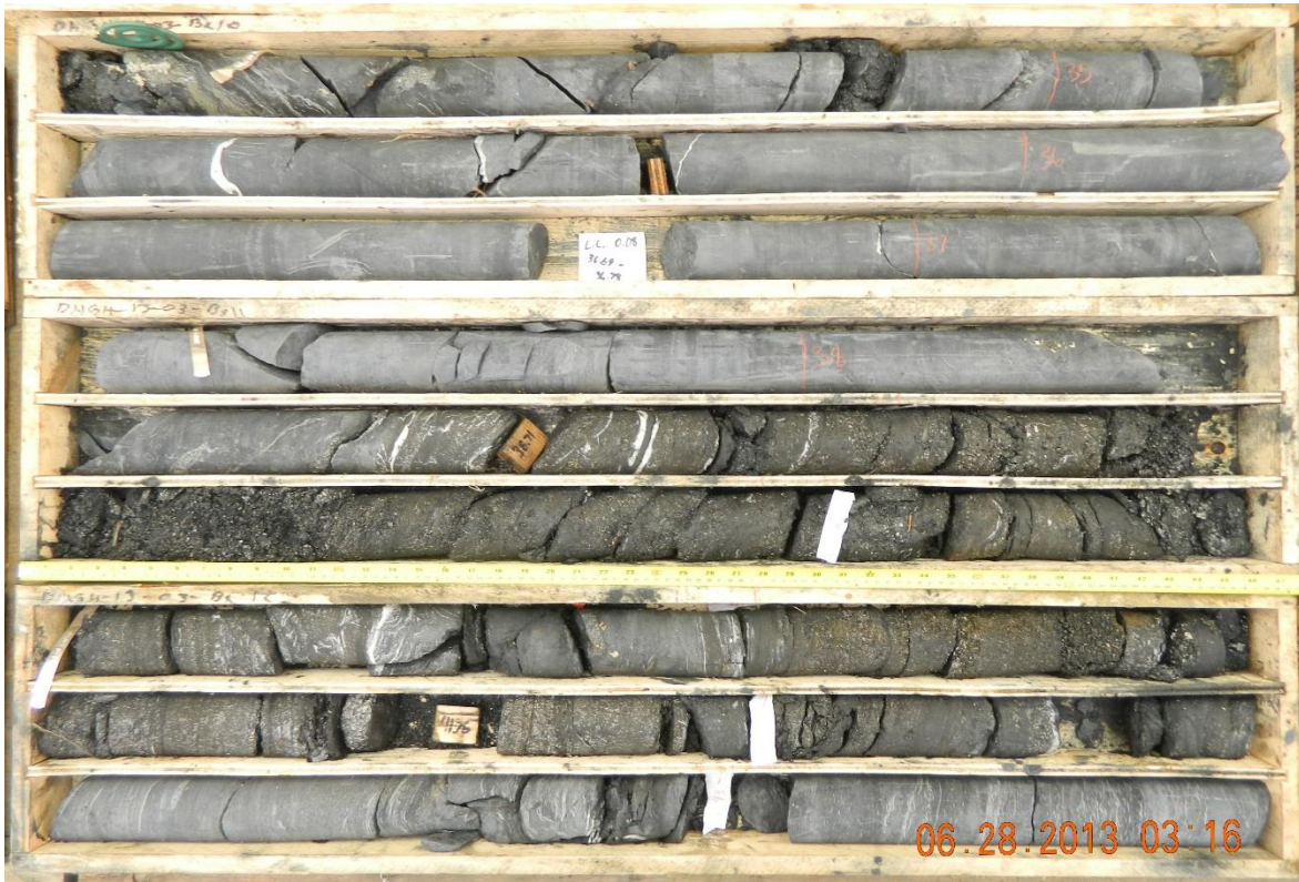
FIGURE 4.5 EXAMPLE OF DISSEMINATED PYRITE AND QUARTZ VEINING WITHIN DHGH13-03
