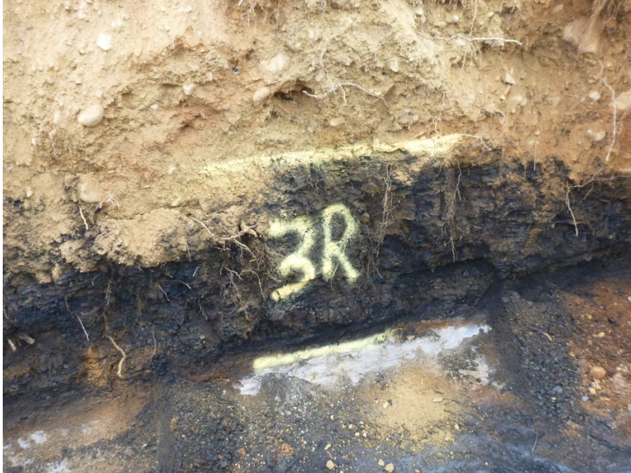
Figure 1: 3R Seam exposed in the rib of the trench, in direct contact with the overlying till
