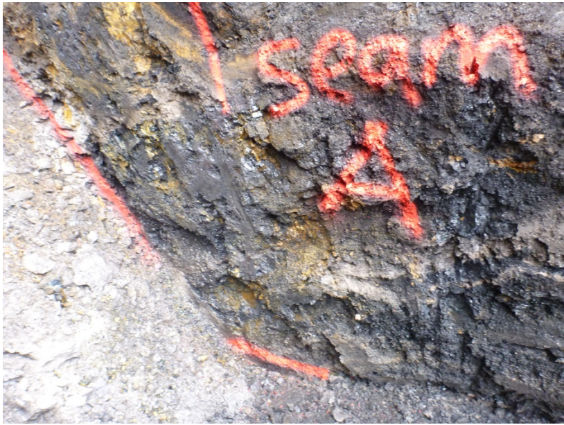
Figure 6: The top part of the 1 Seam, labelled 1 Seam A only for sampling purposes.
