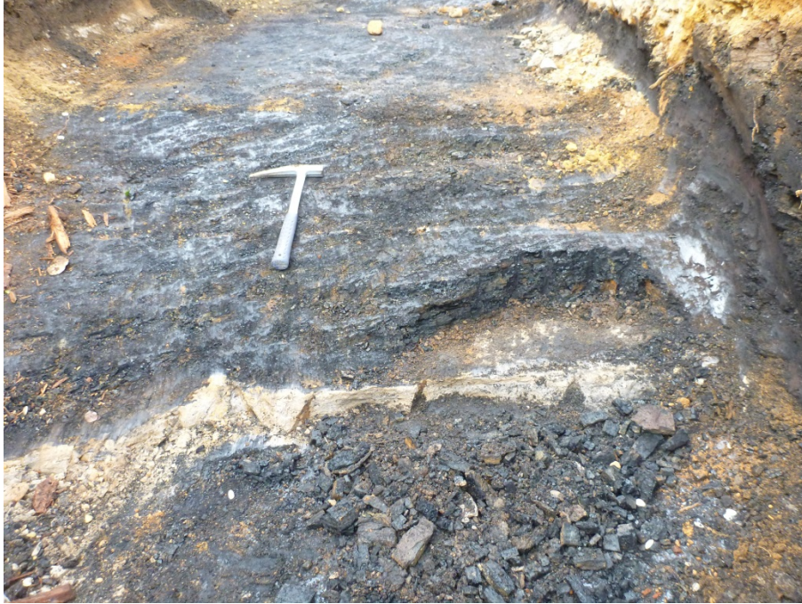
Figure 3: The rock hammer is lying on the top of the #3 coal seam, but also shown in this picture is the top sandstone parting within this seam
