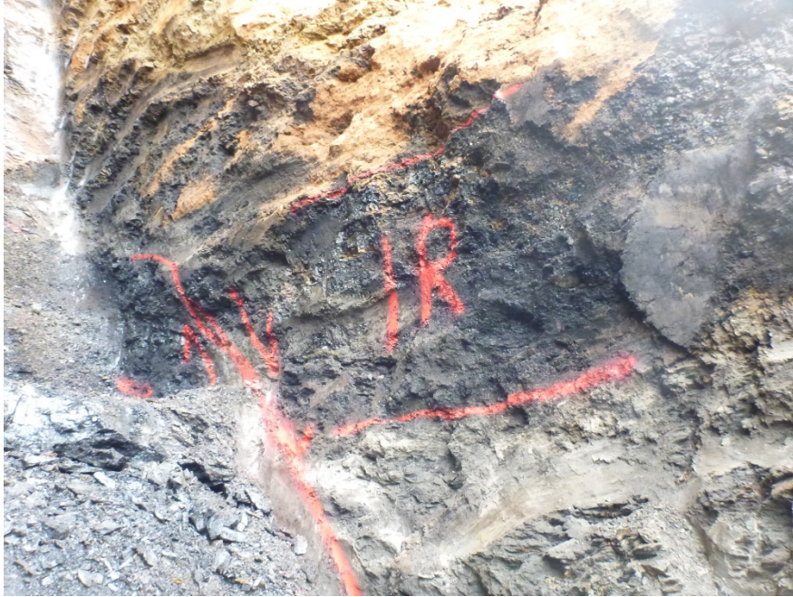
Figure 3: Fault offset through the coal zone, noted mostly through the 1R seam and the 1R-1 Parting
