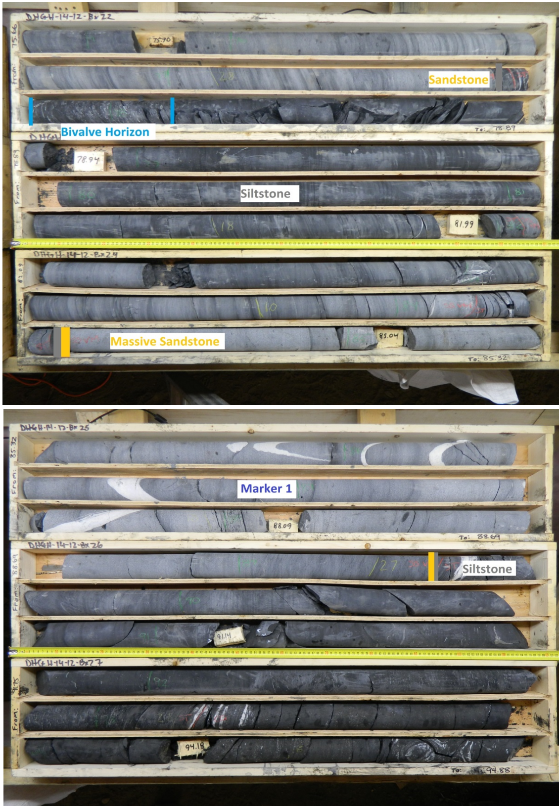
Figure 7. Marker 1 as it appears in core from DHGH-14-12, displaying a clean sandstone with accessory quartz veins. The bivalve horizon is visible above the marker.
