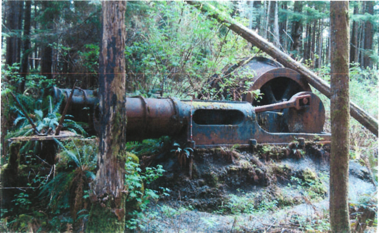
Plate 4: Vulcan Iron Works hoisting engine, in the forest near No.2 Shaft.
