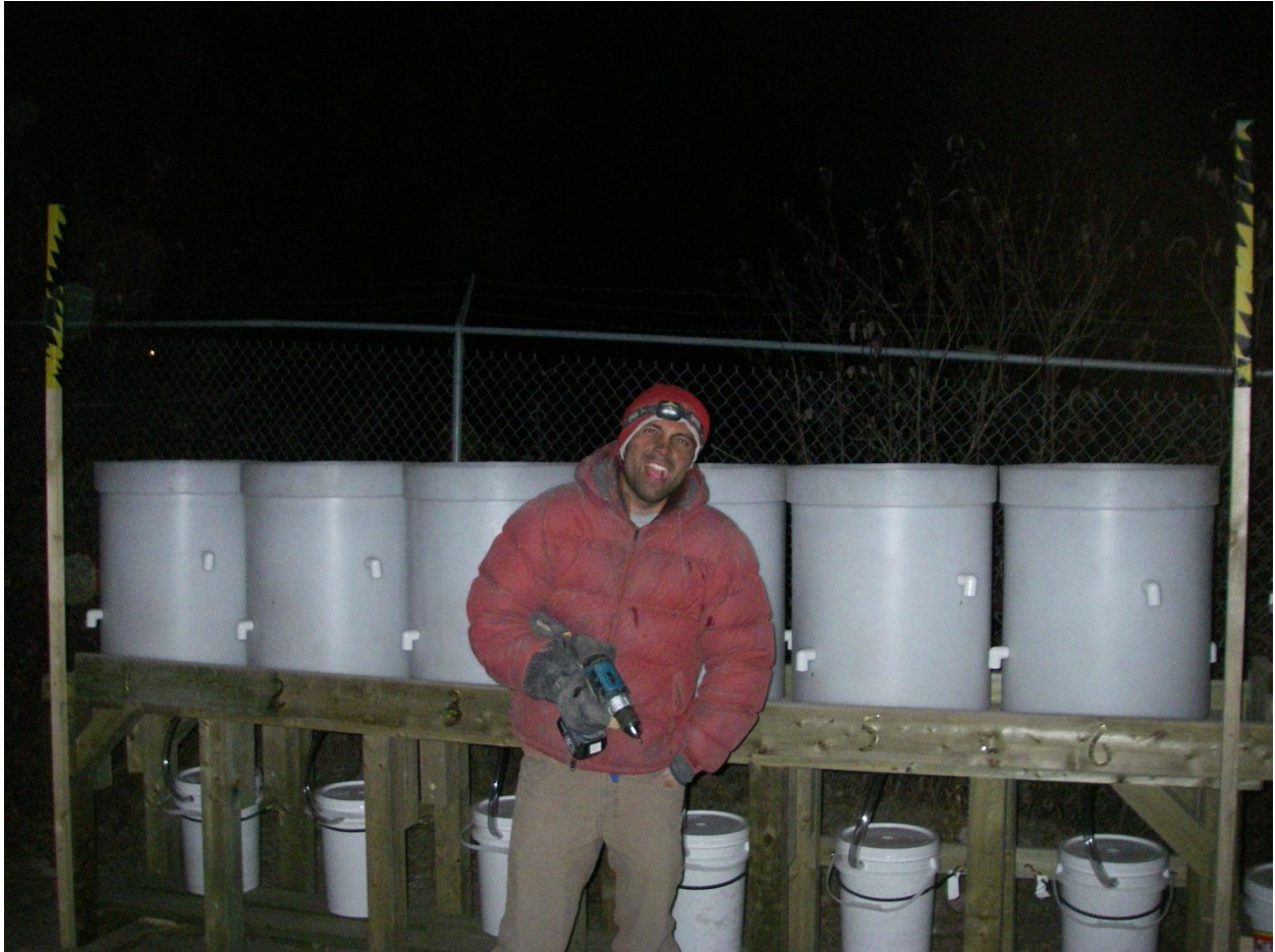
Figure 11: Completed Field Cells with Delineating Uprights with Marking Tape
