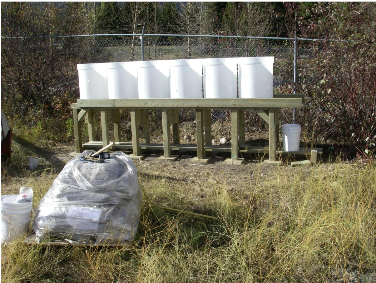
Figure 5: Progression of Working on the Support Structure and Field Cells (Sample Pulps in the Foreground)
