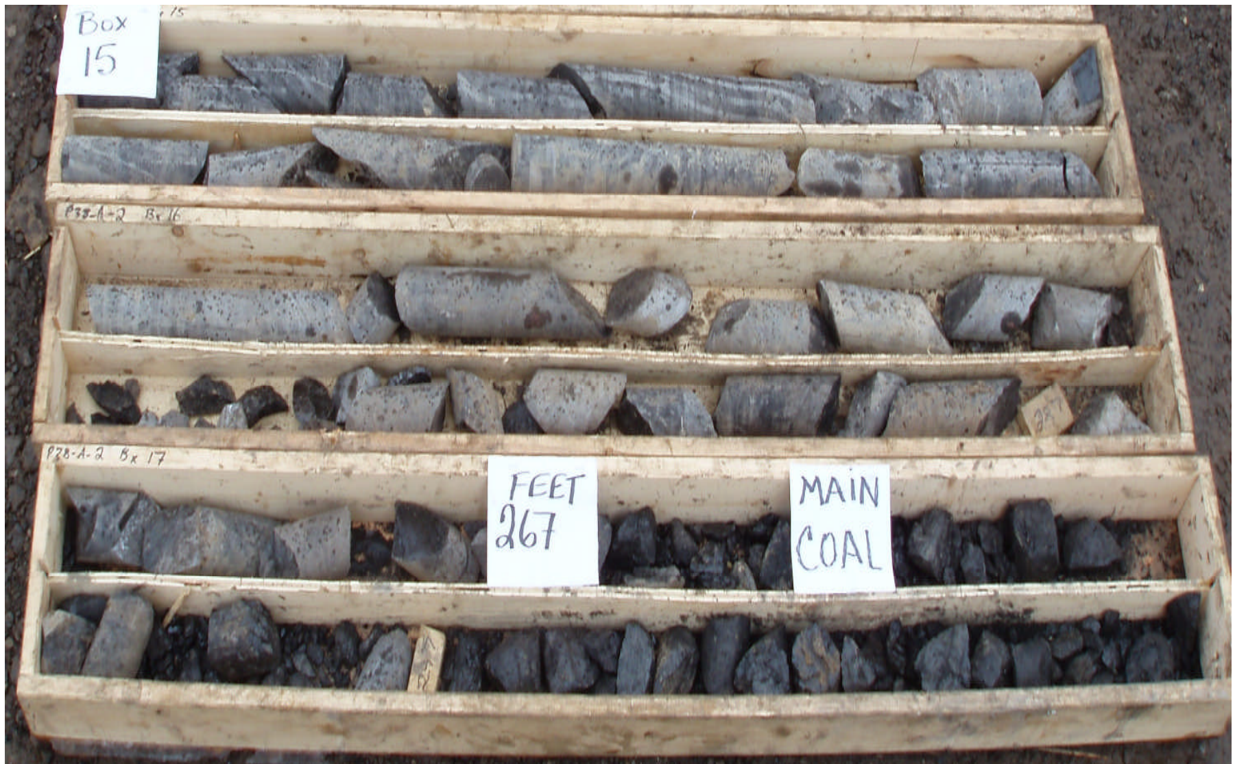
Pic 5: Box 15 to Box 17 (#21L SEAM) TD=307ft.
