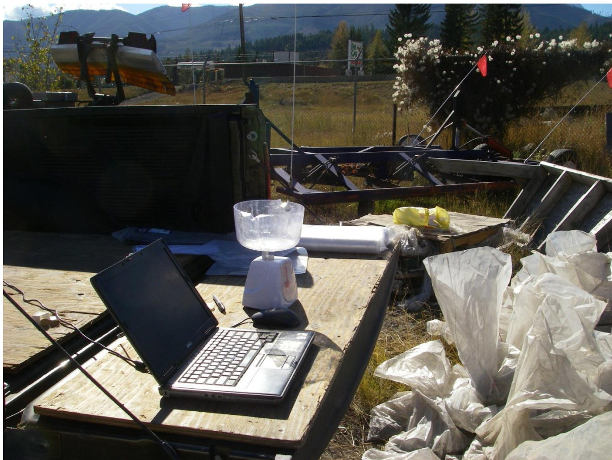
Figure 8: Weighing and Recording Station (Sample Material Seen to Right)
