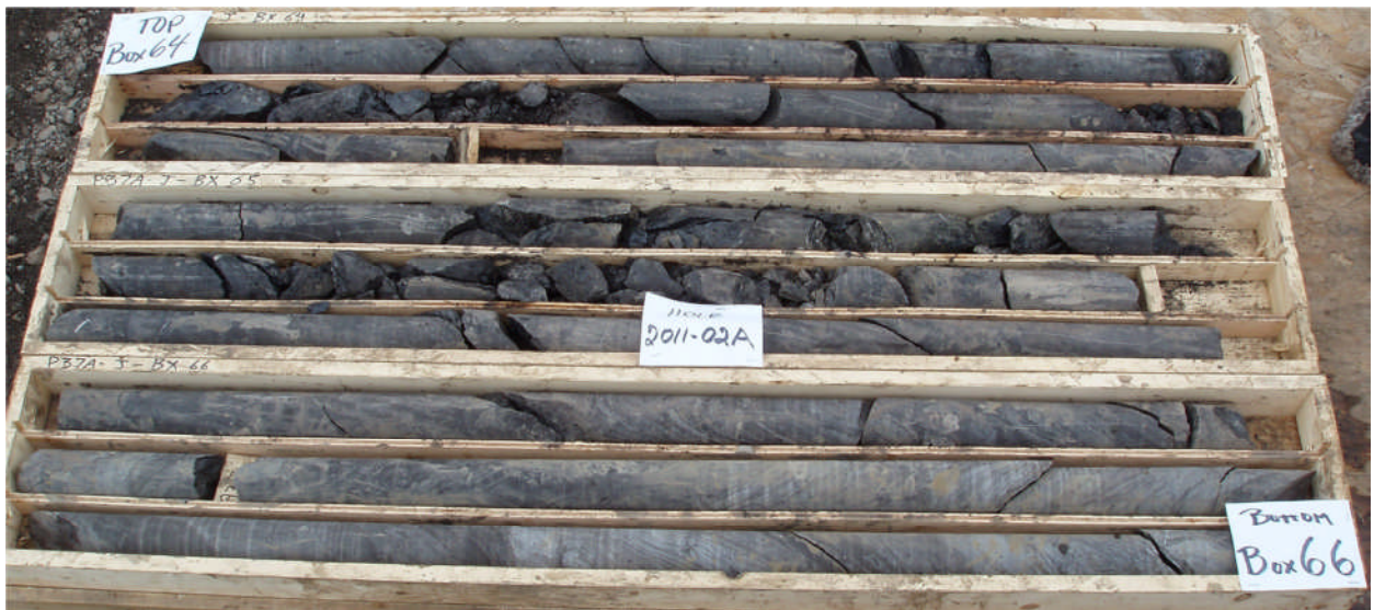
Pic 22: Box 64 to Box 66 (Fracture zone)
