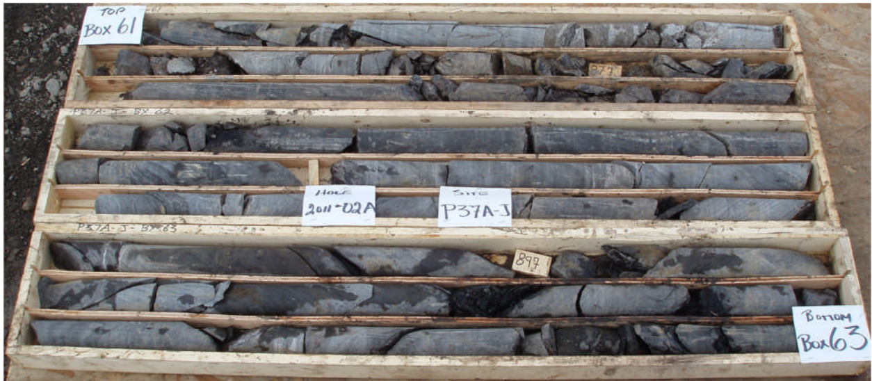
Pic 21: Box 61 to Box 63 (Fracture zone)
