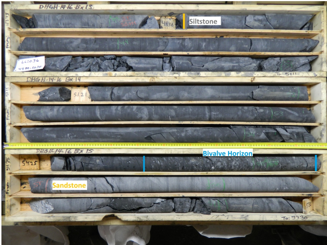
Figure 4.7 Dill core photos from drill hole DHGH-14-16 displaying the three units that comprise a typical Marker 2. The uppermost sandstone is most recognisable by its clean, massive appearance and sharp contact with the underlying siltstone. Following the marker, the bivalve horizon is visible, which further constrains the position of Marker 2.
