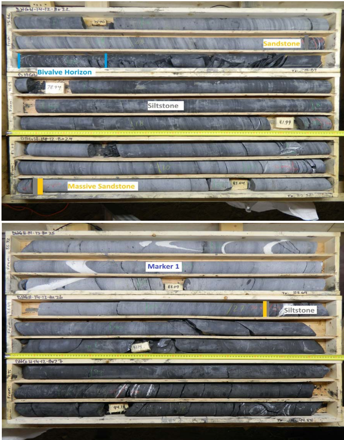
Figure 4.5 Marker 1 as it appears in drill core from drill hole DHGH-14-12, displaying a clean sandstone with accessory quartz veins. The bivalve horizon is visible above the marker.
