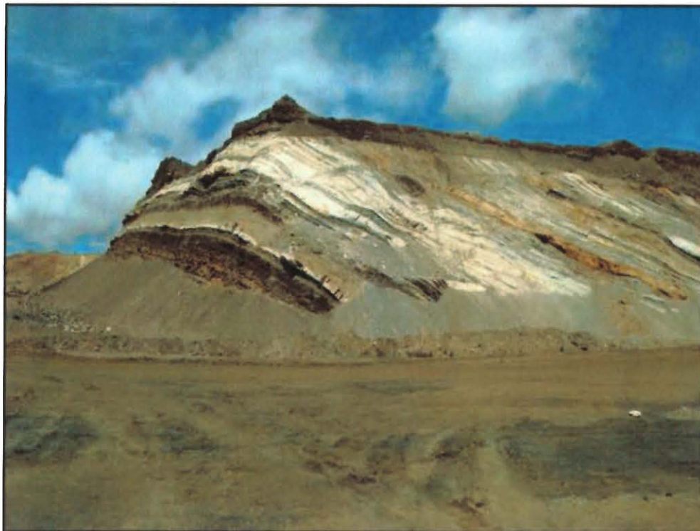
Photo 4: Pit hangingwall where dips are 45 degrees or less, indicating that the seam dip must get shallower with depth.
