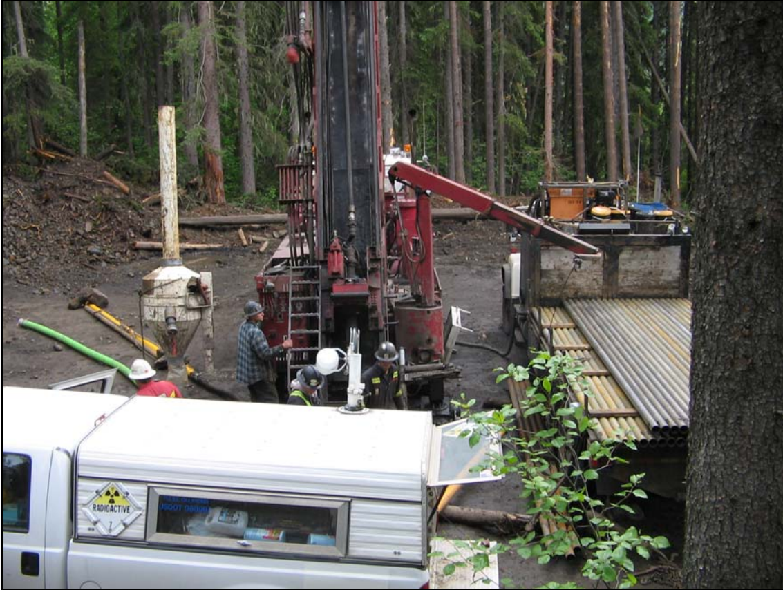
Photo 20: Geophysical logging being performed on site by Century Geophysical
