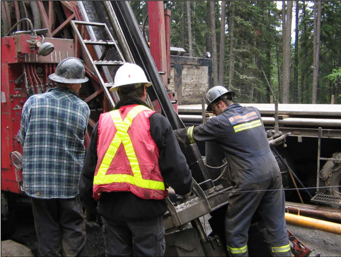
Photo 21: Geophysical logging tool being retrieved by Weatherford Inc. of Grande Prairie
