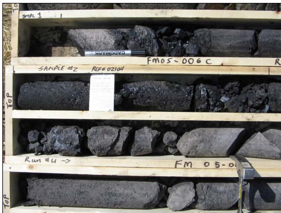
Photo 17: Core box showing core sample with sample tag attached
