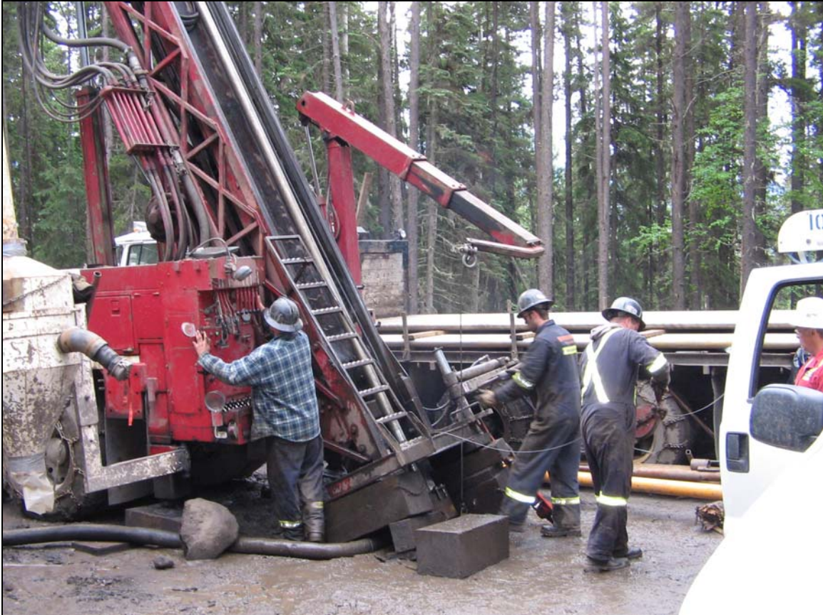
Photo 8: SDS drill crew drilling angle hole
