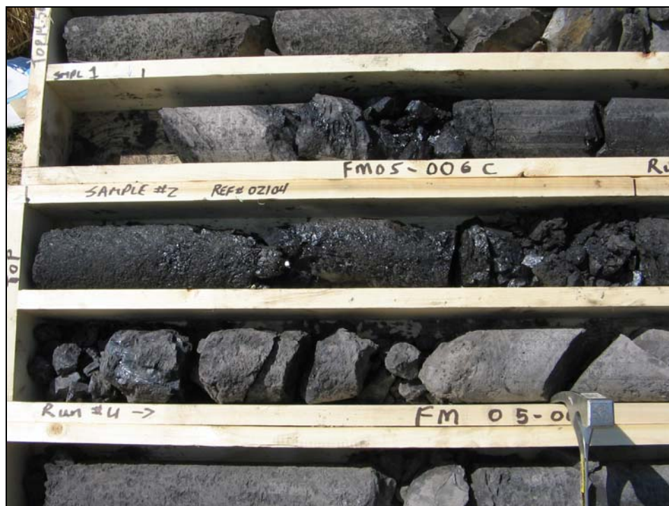
Photo 16: Core box with coal sample marked for removal
