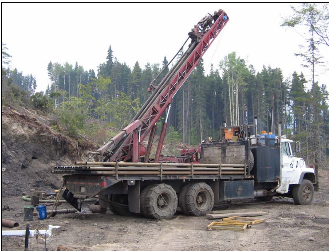
Photo 12: SDS drilling rig set up on angle hole
