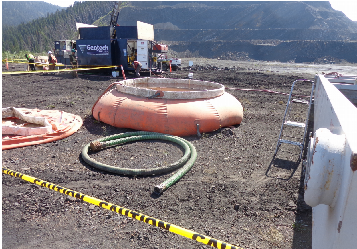
Plate 1: Geotech Drilling Services diamond-drill at site on then-inactive floor of 4N2 open-pit. Orange bladder contains water supply for drilling. Metal structure at extreme right is skid-mounted mud-tank. Southeastern highwall of 4N2 pit is in distance. [RC4927/18.jpg]
