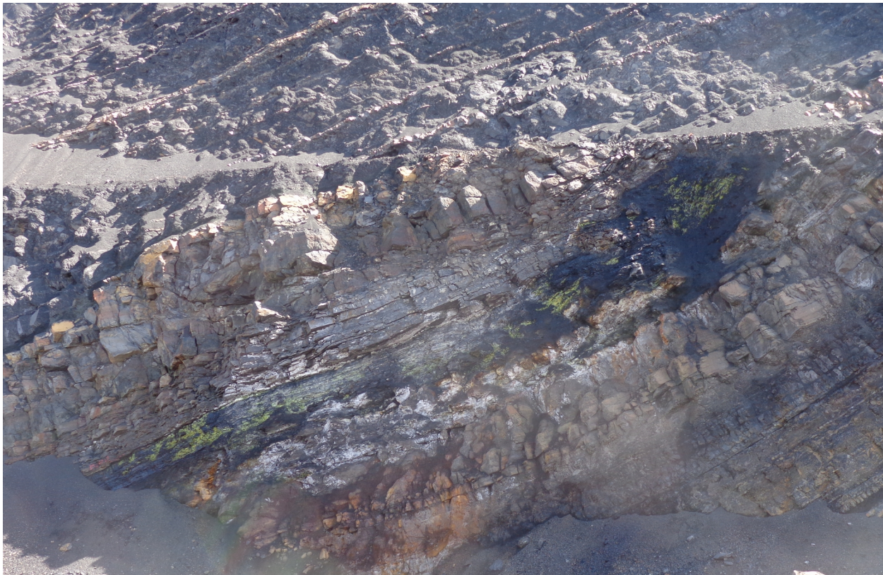
Plate 6: Bird coal seam, approximately a metre thick, as exposed in the southeastern highwall of the 4N2 open-pit workings. Coal seam comprises alternating blocky and sheared mushy bands. Note the bright yellow sulphate bloom on the weathered surface of the coal. Above is about 3 metres of silty sandstone and pebbly sandstone of the uppermost Gaylard Member, in turn erosionally-overlain by dark-weathering Bluesky gritstone. Top of exposed section is Bullmoose siltstone with centimetre- to decimetre-thick bands of conspicuously light-weathering tuff. [RC4841/18.jpg]
