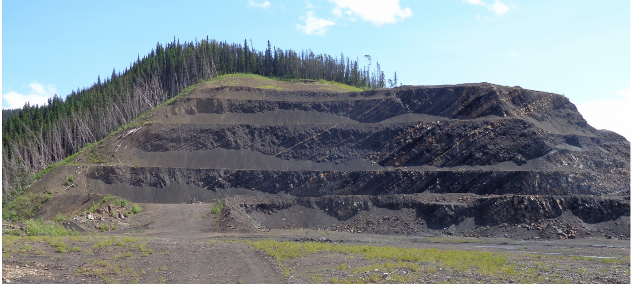
Plate 4: Southeastern highwall of 4N2 pit, as seen prior to resumption of mining in autumn of 2018. Forested slopes are underlain by siltstones with minor bands of ironstone and tuff, of the basal two-thirds of the Bullmoose Member of the Moosebar Formation. Cleared hillside to right is underlain by interbedded siltstone, sandstone, coal and variably-carbonaceous mudstone of the Gaylard Member of the Gething Formation. Closely-associated 400, 401, and 410 coals come to the ridgeline at the extreme right of the photograph. Bedding forms a northeastward homoclinal panel of strata, at dips of 30 to 32 degrees. [RC4849/18.jpg]
