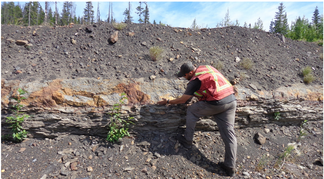
Plate 5: Geologist's hand marks erosional contact of Bluesky pebbly gritstone over Gaylard sandy siltstone. Rusty weathering habit of Bluesky rock suggests potential for acid rock drainage. View is to northeast, along eastern edge of 7S open-pit workings [RC4945/18.jpg]
