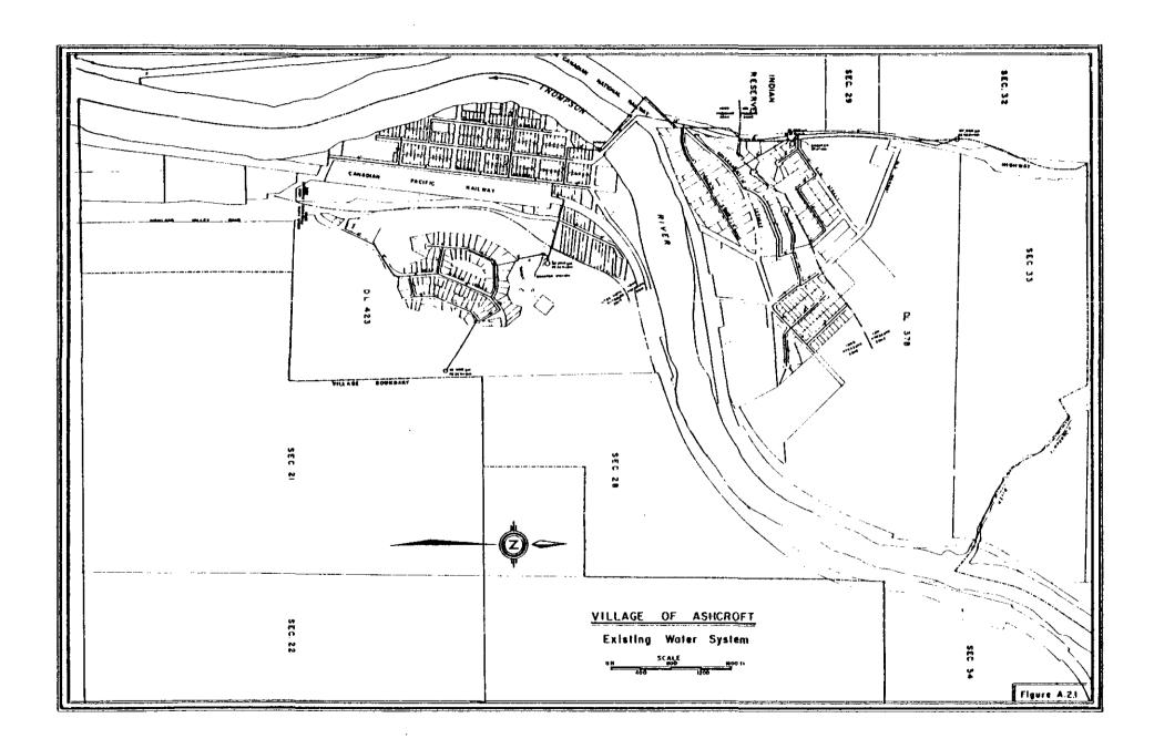
in both North and South Ashcroft are in hydraulic balance thereby enabling simultaneous pumping from the intake into both reservoirs. Booster stations at the lower reservoirs pump water to the higher pressure zone in both North and South Ashcroft.
