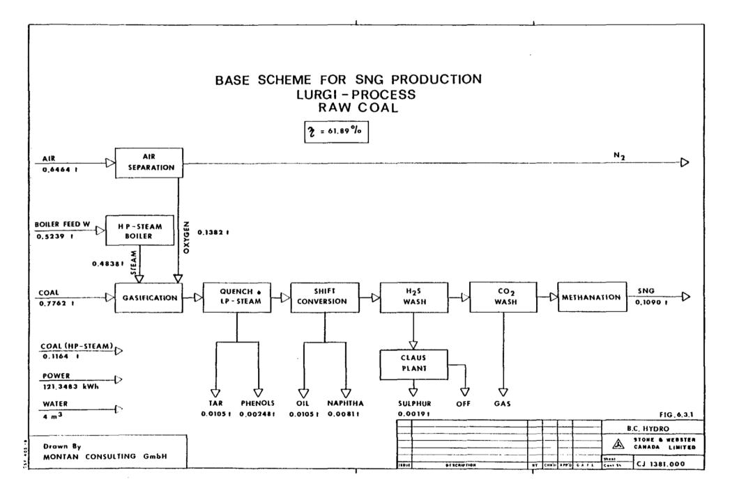
6.3.1.6 A materials balance and overall thermal efficiency for washed coal is shown in Fig. 6.3.2 based on It of raw coal feed.
