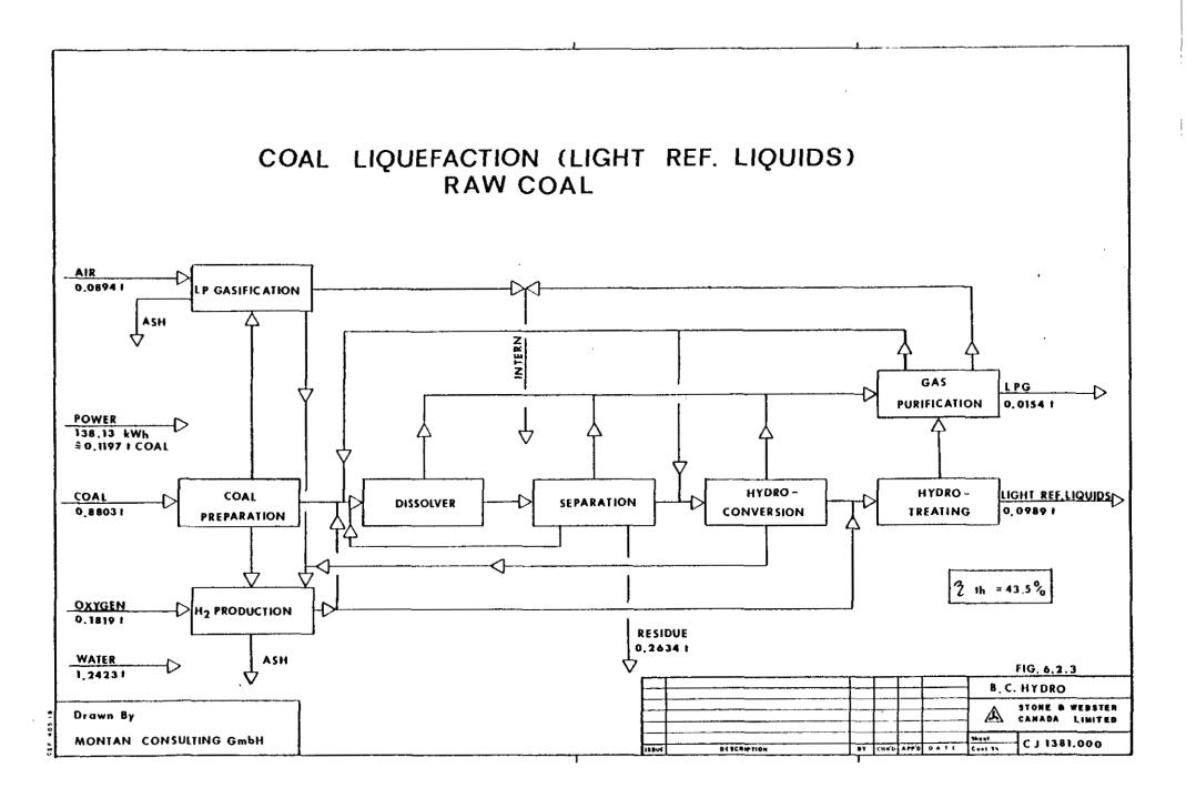
6.2.2.3 A materials balance and overall thermal efficiency is shown in Fig. 6.2.4 for washed coal feed.
