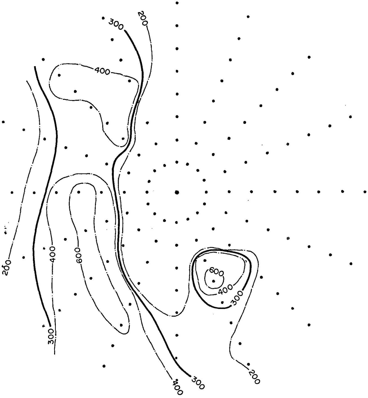
Figure F6-11 PREDICTED ANNUAL MAXIMUM 3-HOUR SO 2 CONCENTRATIONS (µg/m 3 ) 366 m STACK WITH MCS
