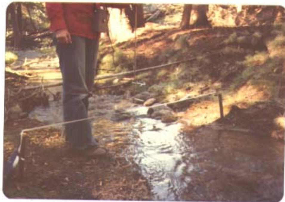
FIGURE B2-2: (76-4-28) Ott propeller-type current meter, ready for streamgauging in Ambusten Creek,
