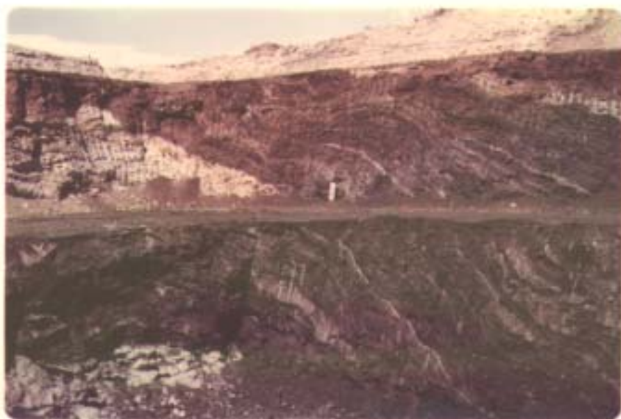
North wall of west end of Trench A. Coal. Note the clearly oxidized zone (brown) cutting across the coal layers under the till. This indicates pre-glacial weathering, not burning.
