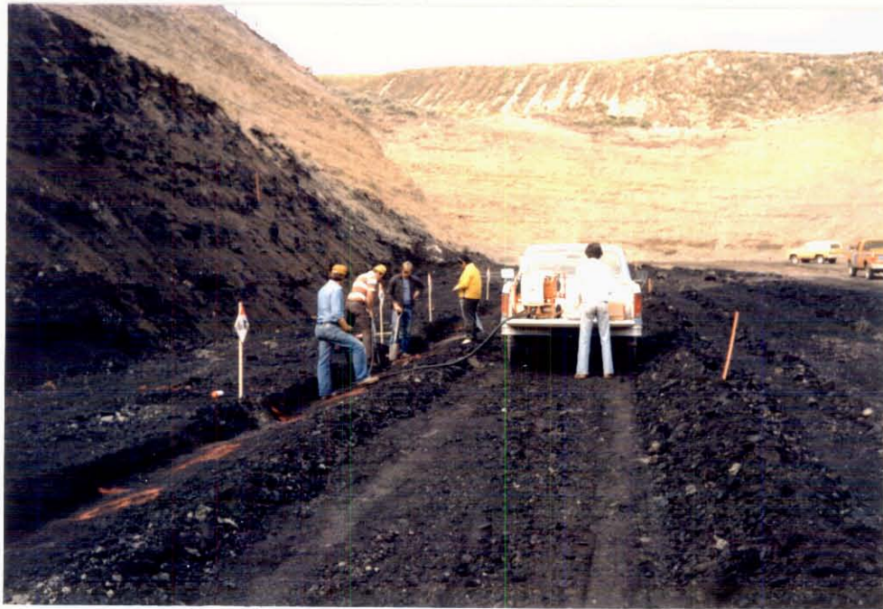
Photo 1: Channel sampling prior to mining the coal.
