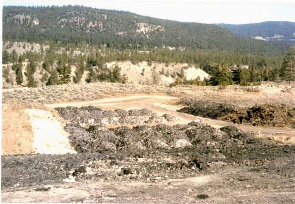
Photo 10: Each clay parting >2 m wide placed in separate row piles.
