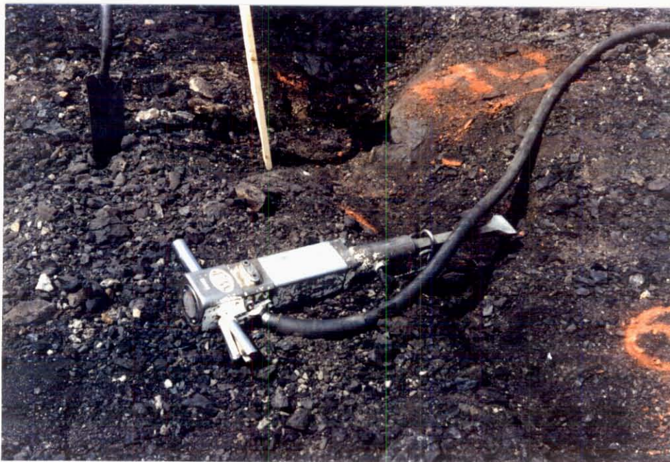
Photo 2: Hydraulic percussion hammer for channel sampling.
