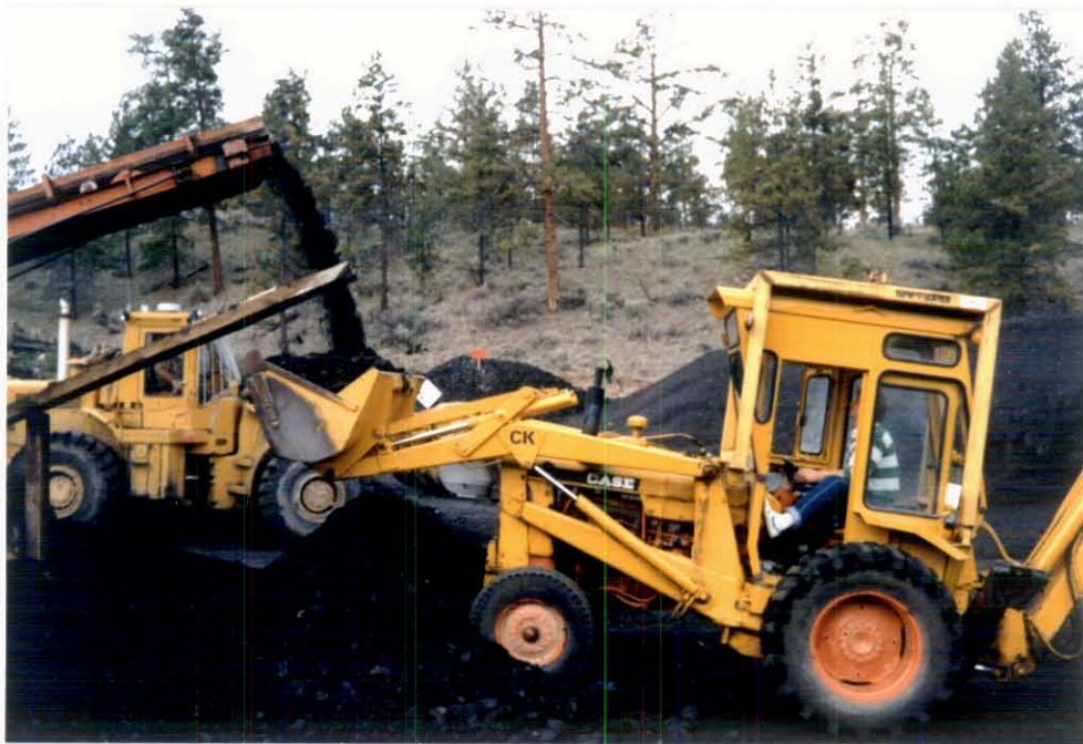
Photo 13: Taking sample cuts with the small backhoe bucket.
