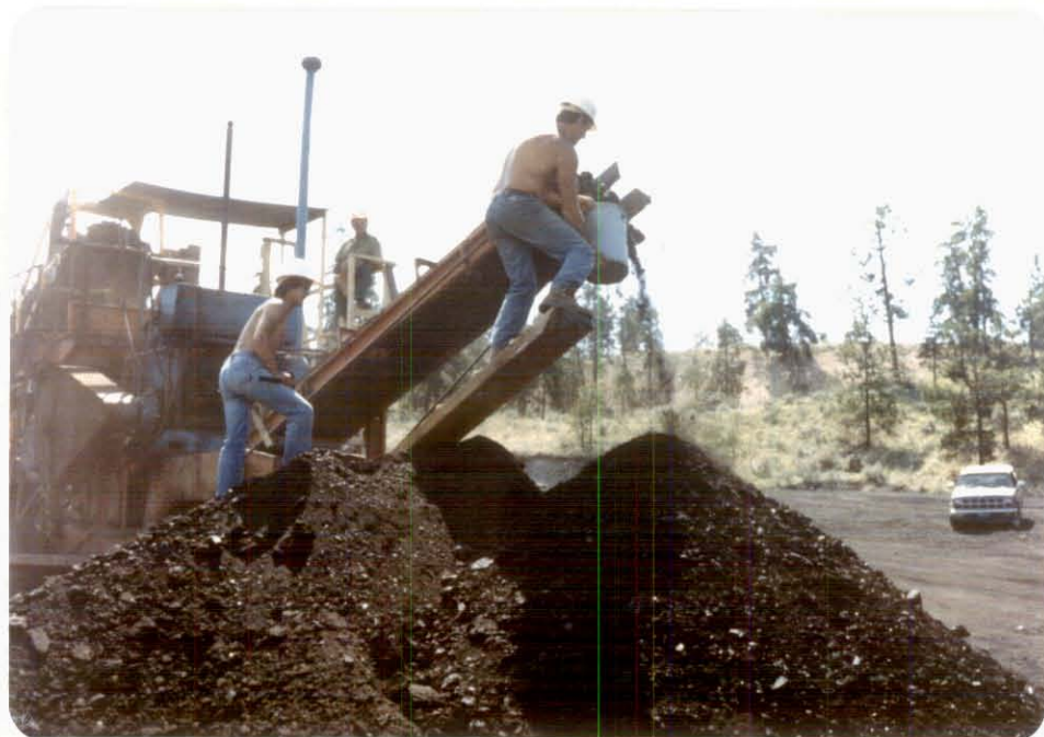
Photo 12: Taking the periodic coal cut laboratory samples.
