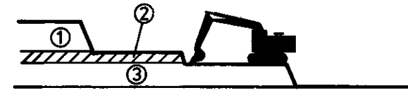
c). Ramp down and use hydraulic shovel to clear parting ②
