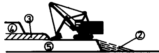
b). Move large shovel onto parting ③ and load parting.
