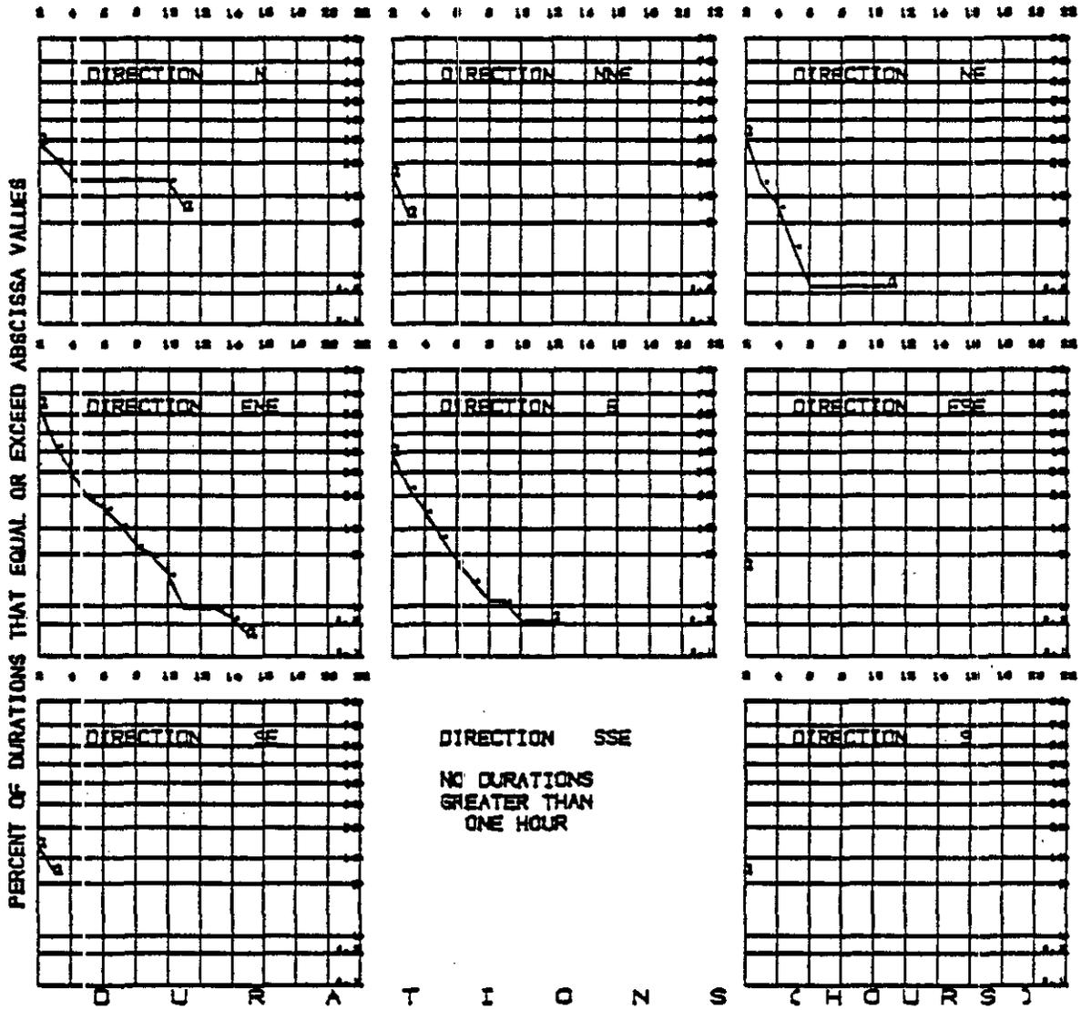
Figure E4-4 Plots of Wind Direction Persistence Versus Frequency for Station 1, Lower Hat Creek Valley
