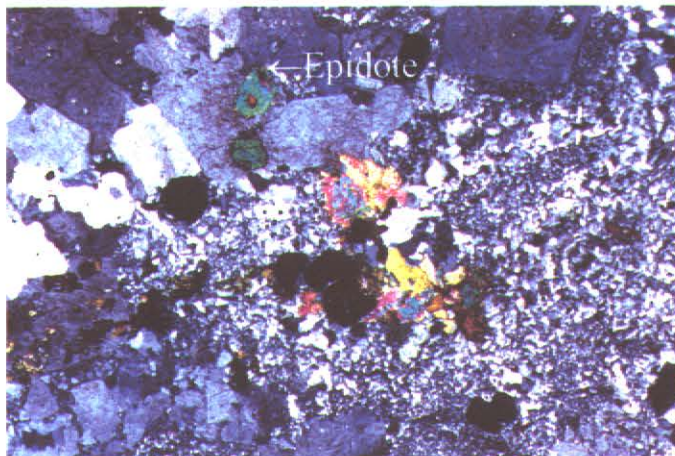
Left: Epidote in fine-grained quartzofeldspathic matrix (width of field = 3.3 mm; crossed polars). Right: Chlorite (dark green) surrounding sieve-textured plagioclase phenocrysts (width of field = 6.6 mm; crossed polars).
