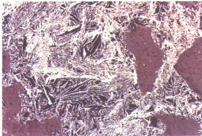
Left: Breccia texture: porphyritic wallrock clasts cemented by hematite (black; width of field = 6.6 mm; crossed polars).
