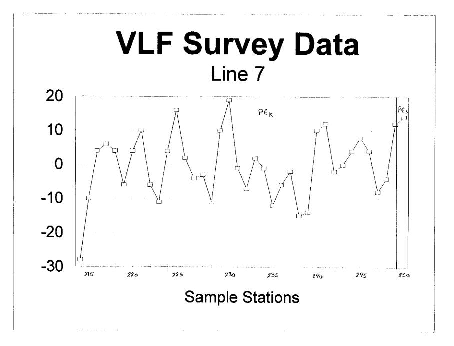
The resulting data was Fraser Filtered and plotted in a series of profiles (Figures). Geological contacts (stratigraphic and structural) have been plotted on the figures for interpretive purposes.
