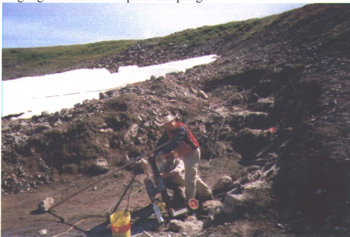
Angling core drill for in place sampling
