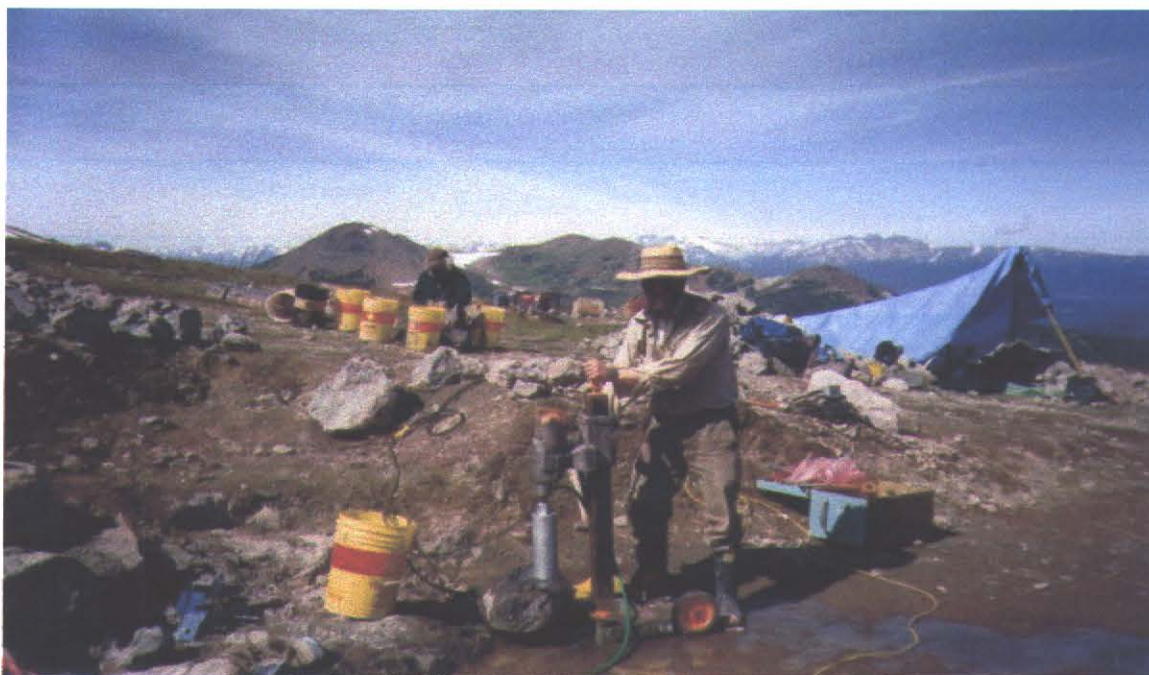
Angling core drill for in place sampling
