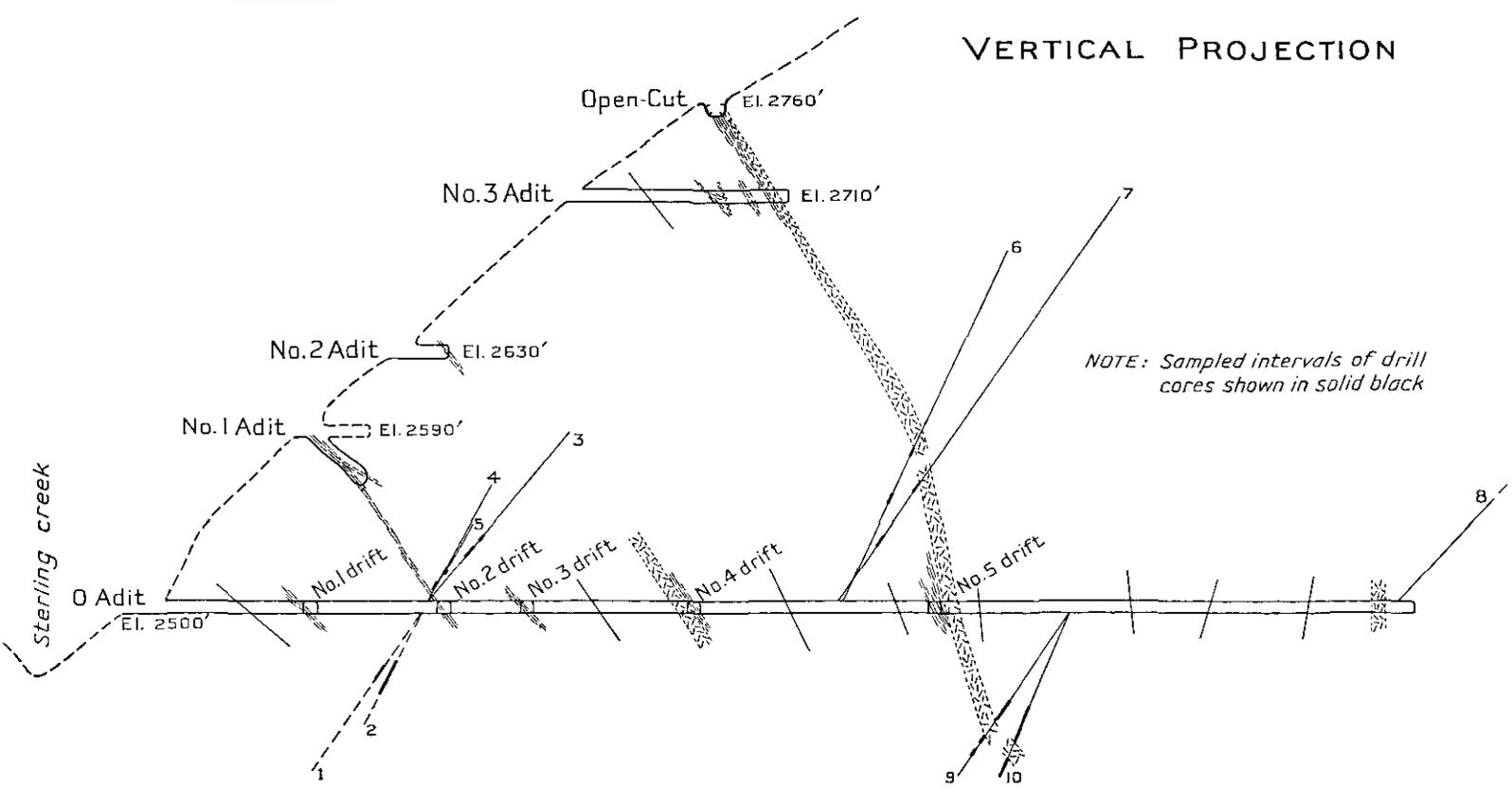
Hedley Sterling Gold Mines, Ltd., Patsy No. 2 workings. Plan and vertical projection on line of "O" adit, from compass survey.
