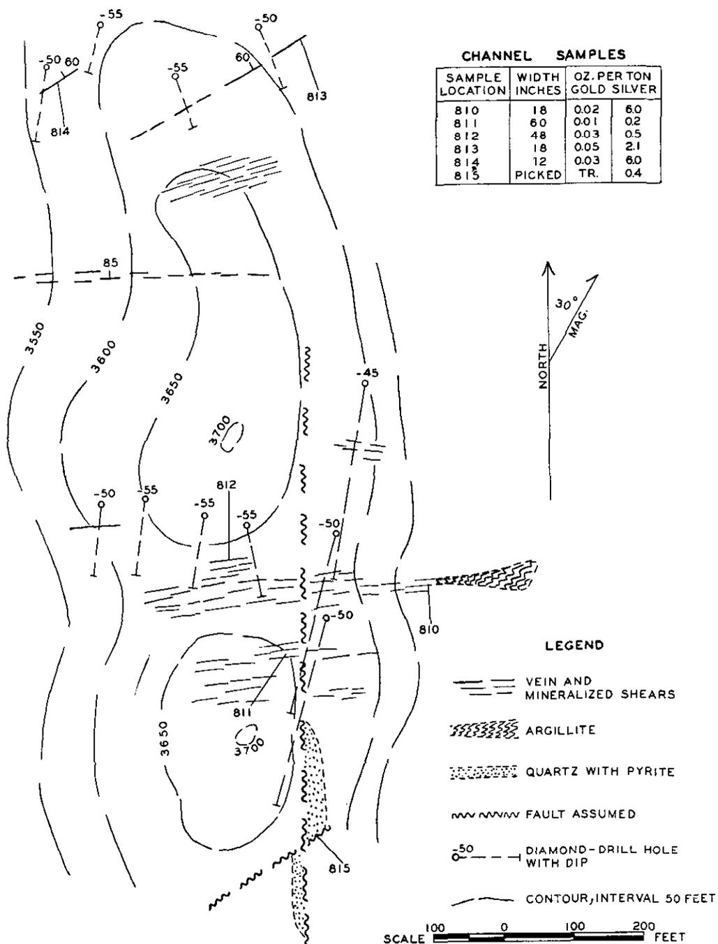
Fig. 7. Cassiar Rainbow Gold Mines, Limited—plan of surface, showing veins, shears, diamond-drill holes, and assays.
