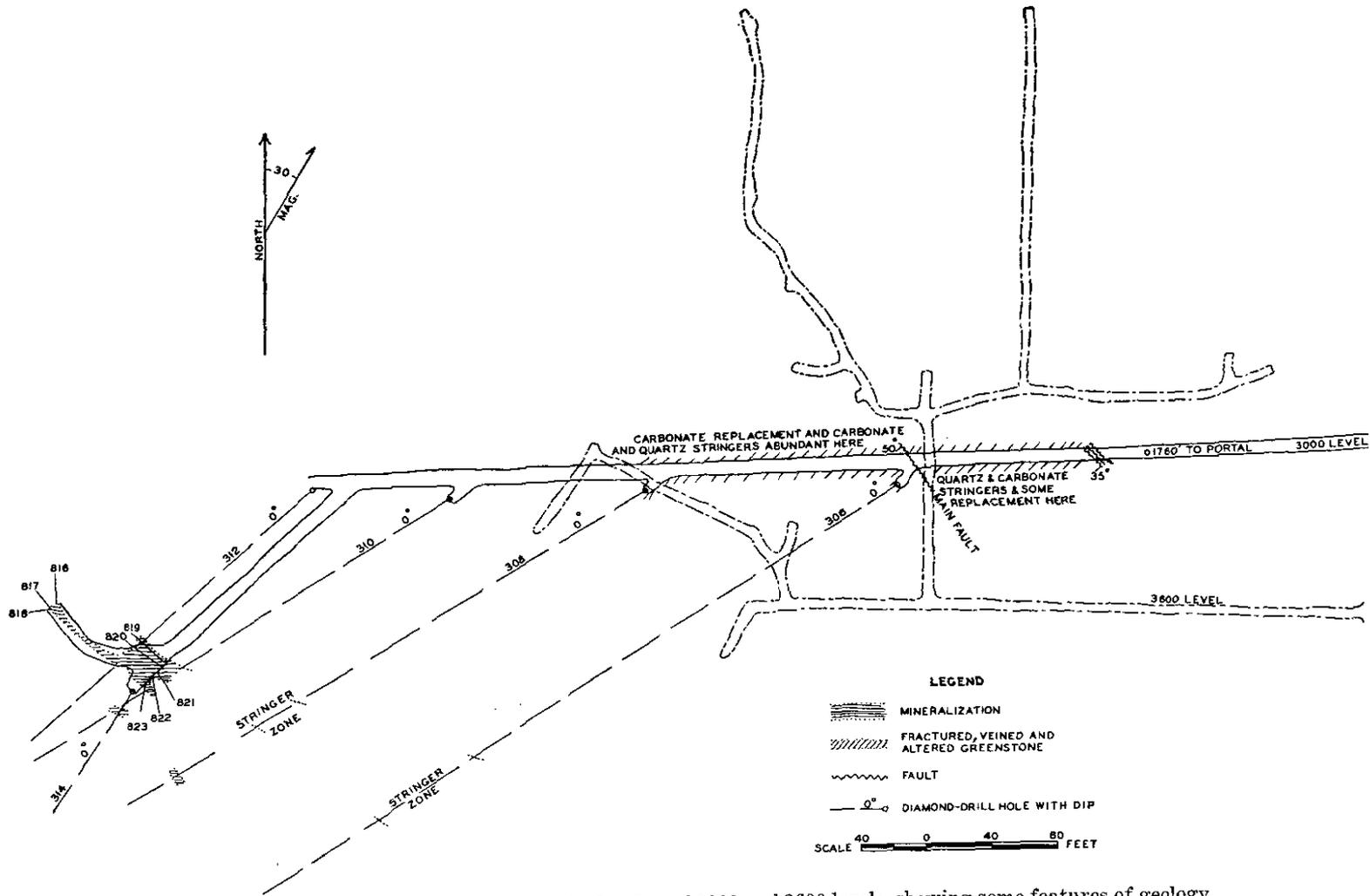
Fig. 6. Morris Summit Gold Mines, Limited—plan of 3000 and 3600 levels, showing some features of geology, mineralization, and the location of samples.
