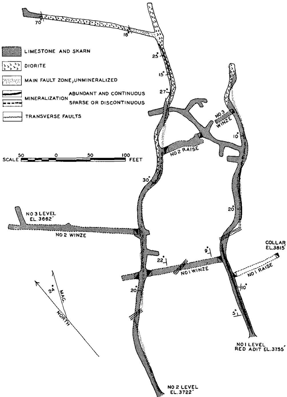
Fig. 19. Hedley Amalgamated Gold Mines, Limited—plan of No. 1 and No. 2 levels.
