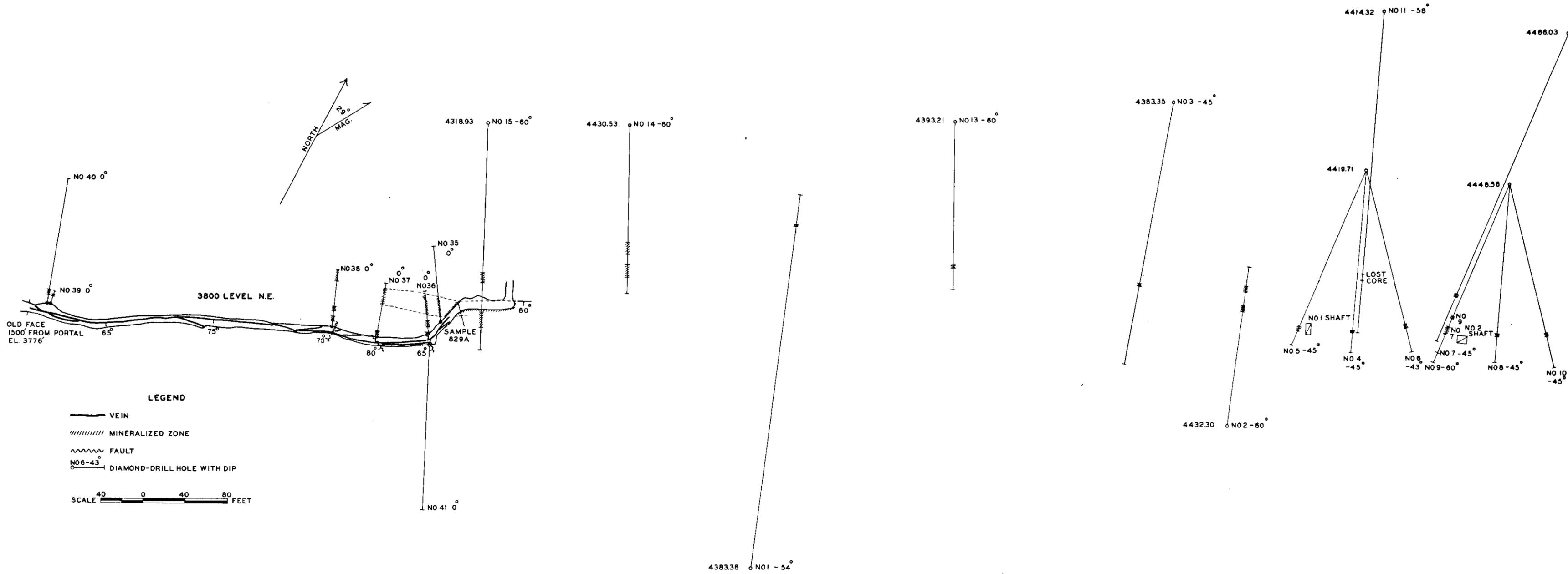
FIG.9. DUTHIE MINE. SHOWING PART OF THE 3800 LEVEL, MINERALIZATION AND DIAMOND-DRILL HOLES
