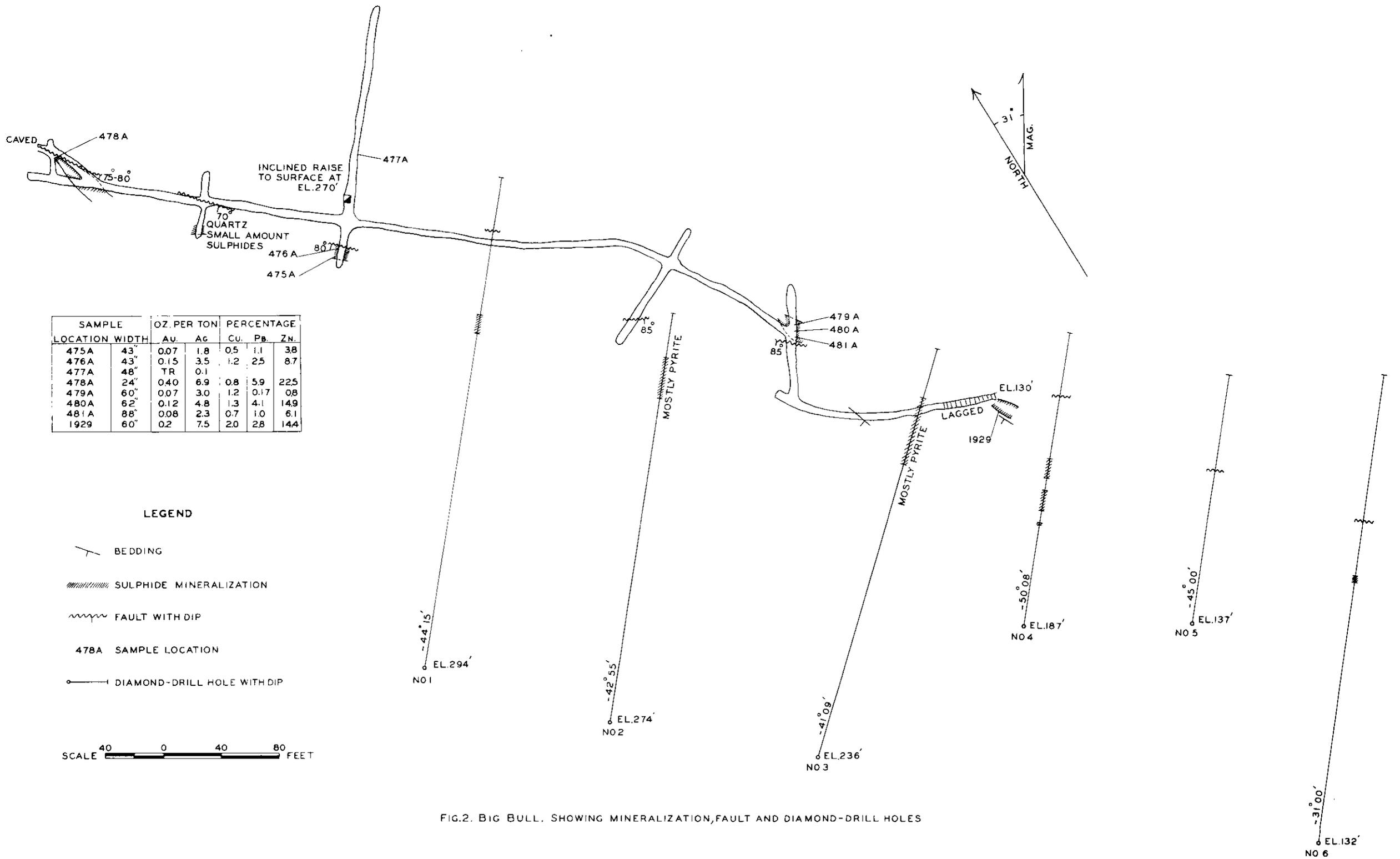
FIG. 2. BIG BULL. SHOWING MINERALIZATION, FAULT AND DIAMOND-DRILL HOLES
