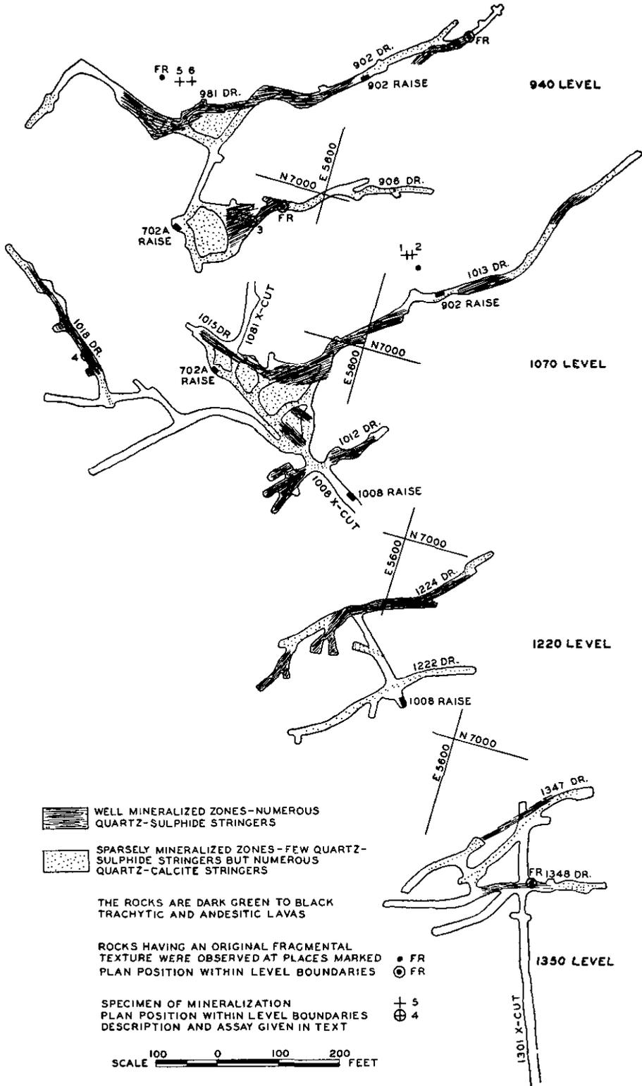
Fig. 5. Silbak Premier mine—plans of 1350, 1220, 1070, and 940 levels in west ore-zone.
