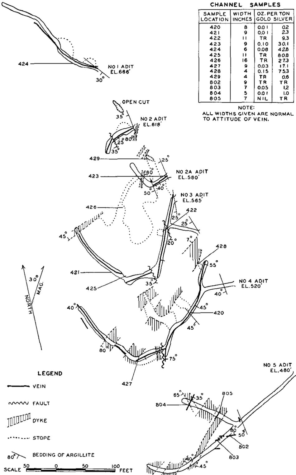
Fig. 8. Esperanza Mines, Limited—plan showing underground workings, geology, veins, and assays.
