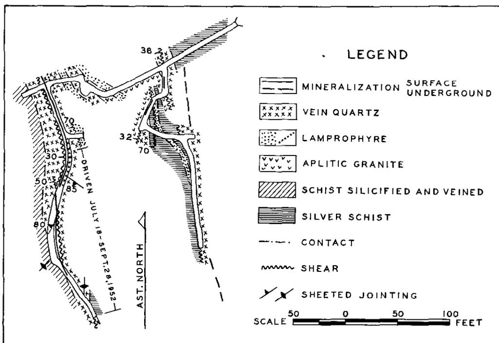
Figure 9. Geological plan of Townsite mine.
