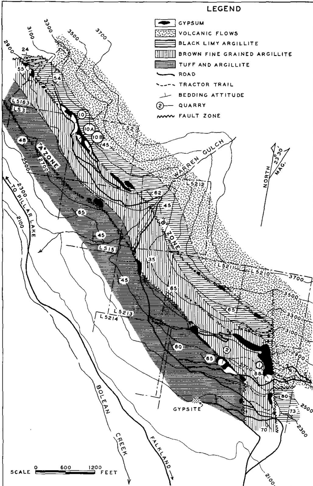
Figure 24. Geology of Falkland gypsum deposit.
