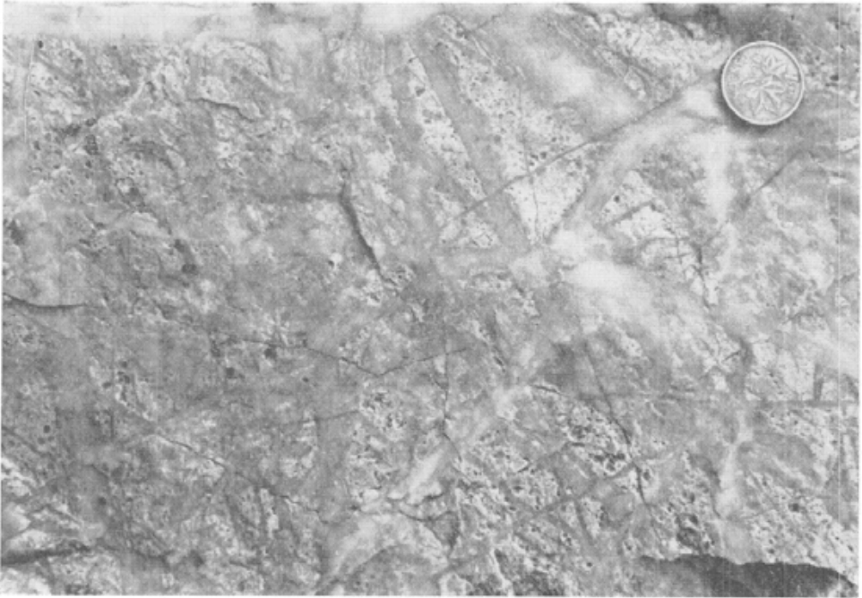
Plate IIA. Quartz-filled stockwork and associated silicification at the Lucky Ship. Mineralized stockworks such as this are typical of many molybdenum and copper-molybdenum deposits in the Central Interior.
