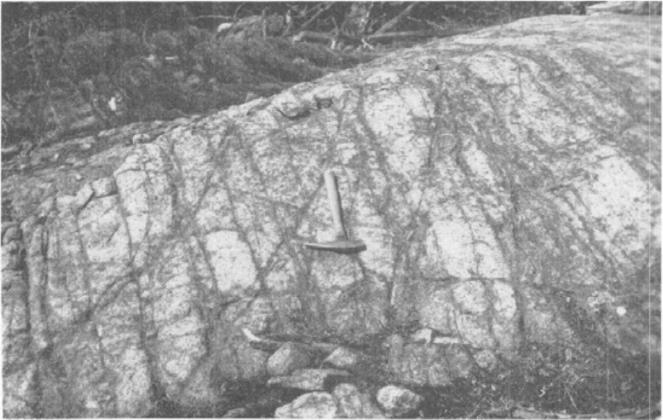
Plate IIB. Surface outcrop of the Brenda orebody showing mineralized fractures in quartz diorite.
