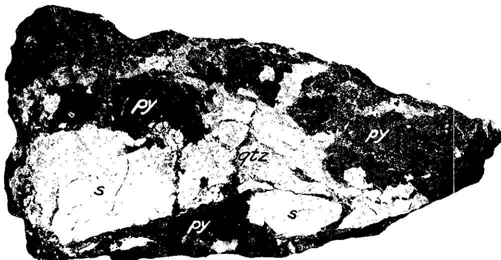
Plate V A Regal Silver. Fractured scheelite (s) with quartz (qtz) and pyrite (py). The distribution of the scheelite is approximately parallel to wall of enclosing pyrite lens. Natural size.
