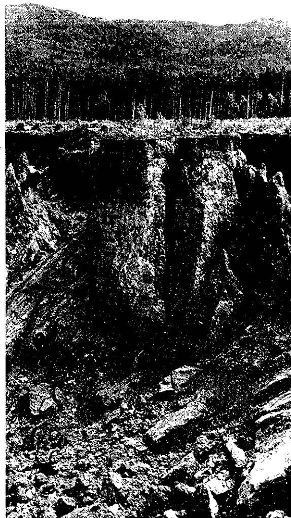
Plate VIII B. A cave at the head of a hydraulic pit showing the large masses into which the boulder-clay breaks.
