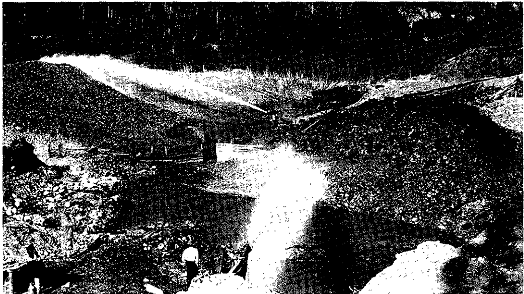
Plate VI B. A hydraulic pit with one giant feeding gravel to a short length of sluce-boxes and a second monitor stacking the coarse gravel at the end of the boxes. Sand and water run off through a sluce-flume to the right.
