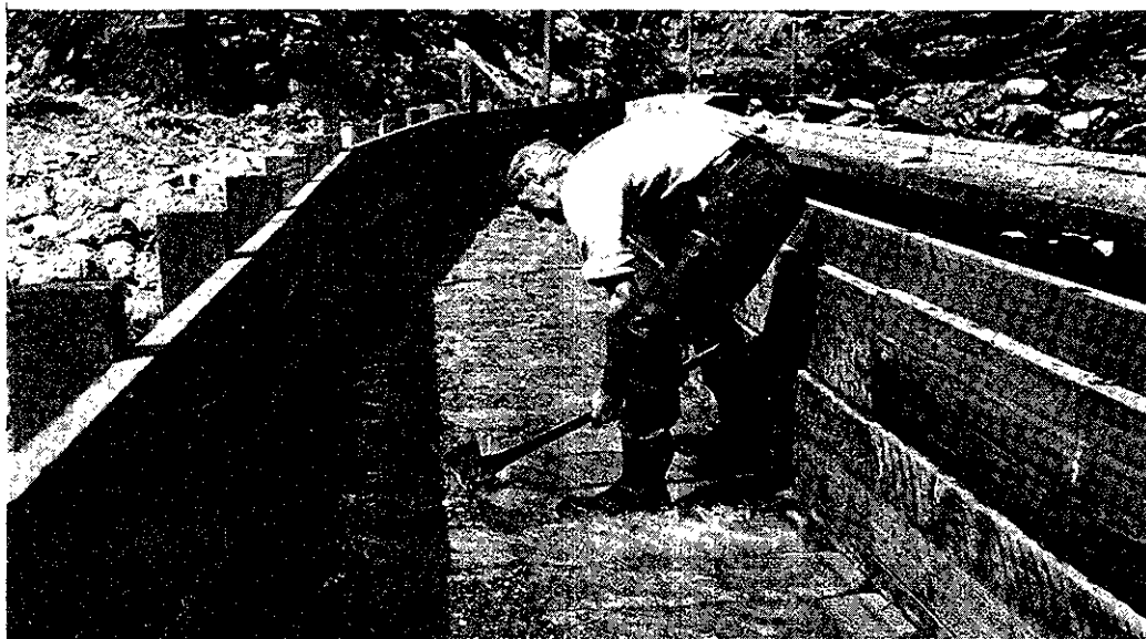
Plate XII A. Loosening up the sand and gravel packed between block riffles.
