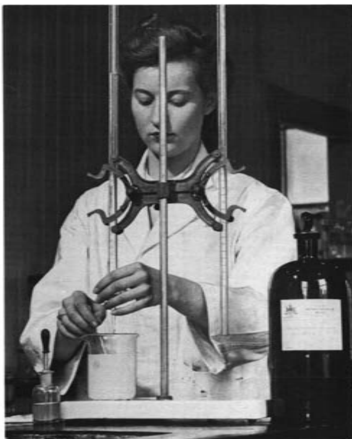
A.—Titration of the zinc solution.
