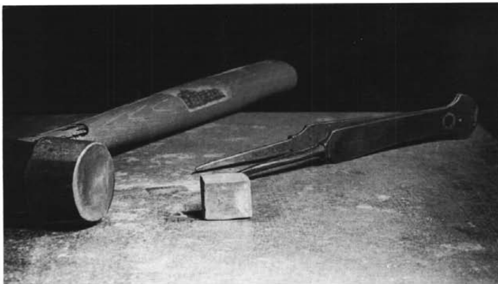
B.—The lead button containing all the precious metals, after the slag has been hammered from it and discarded.
