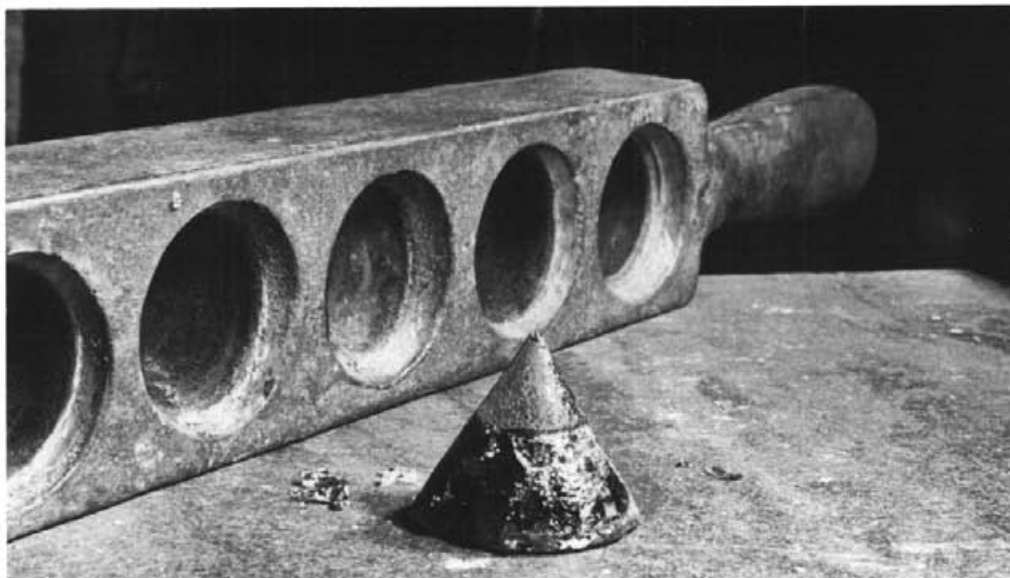
A.—Cooled slag with lead button attached.
