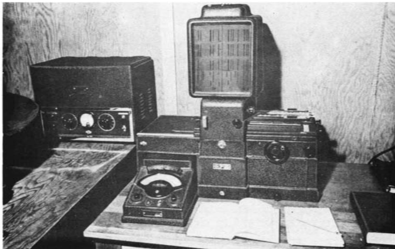
A comparator used for reading spectrograms, and a densitometer used for measuring the blackness of the lines.
