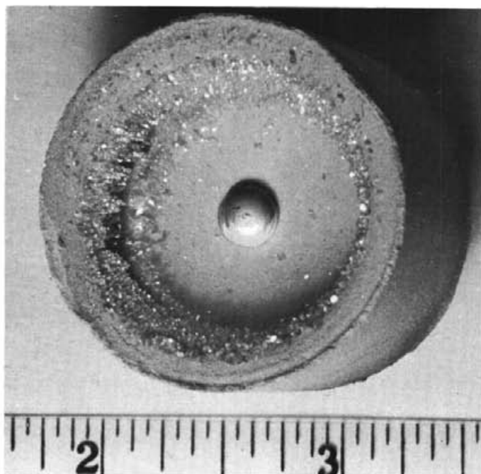
B.—A cupel with an exceptionally large silver bead remaining at the completion of the cupellation process.
