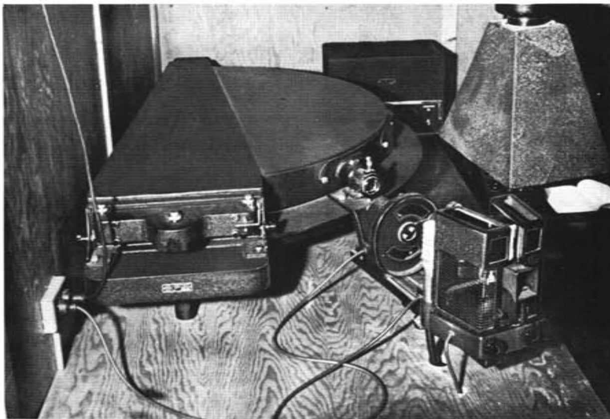
The spectrograph, an instrument to analyse and photograph the light emitted by incandescent metallic vapours. An electric arc produces these vapours from the powdered rock. The arc is enclosed in a wire cage shown on the right. The camera is on the left. The instrument is about 5 feet long.
