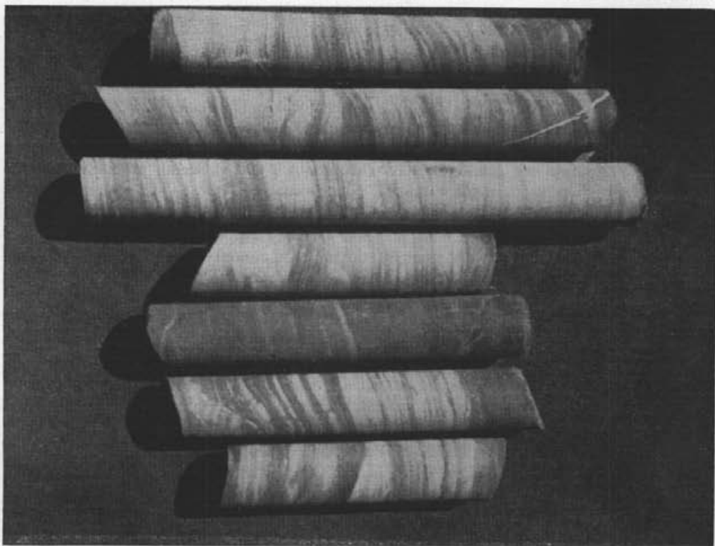
Plate VI. Finely bedded silty rocks in diamond-drill core from Lookout crosscut.
