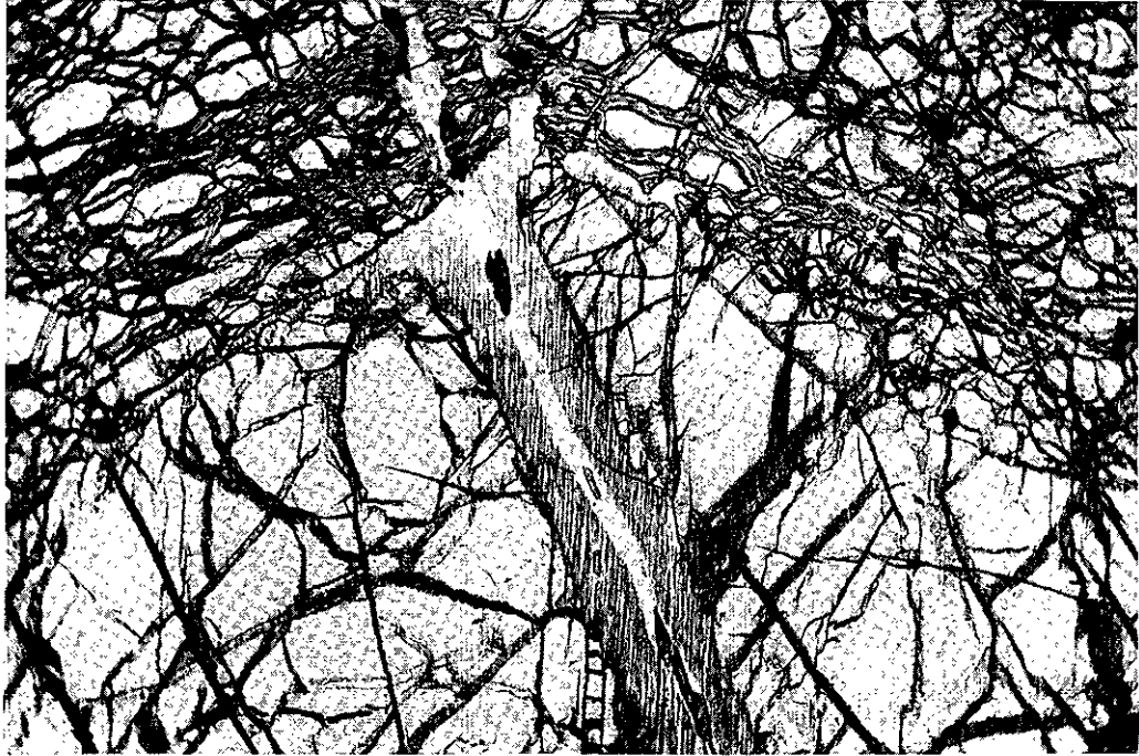
Plate X. Uneven advance of serpentinization from a fracture in a large enstatite grain that contains diopsidic lamellæ (see Plate XI). The lamellæ are relatively resistant to serpentinization and project into the serpentinized part; the material above the enstatite is partly serpentinized olivine; magnification, \times 78 .
