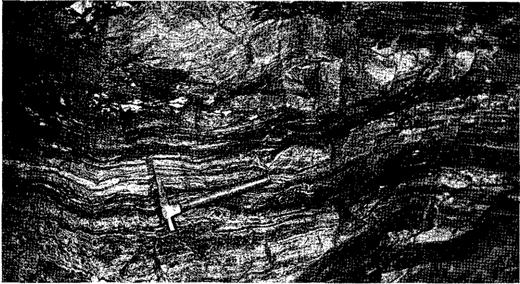
Banded zinc ore in the B zone, Jersey mine; sulphides, mainly sphalerite, dark grey; dolomite, light grey and white.
