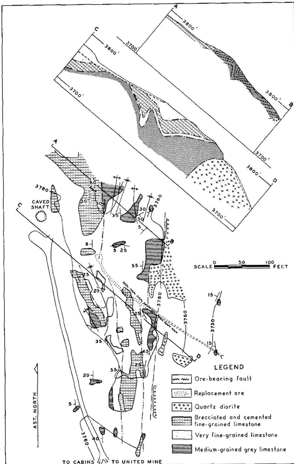
Figure 29. Geological plan and section of the Star mine.
