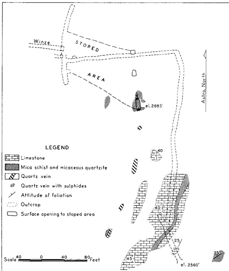
Figure 18. Surface geology and underground workings, Eden and Crescent mine.
