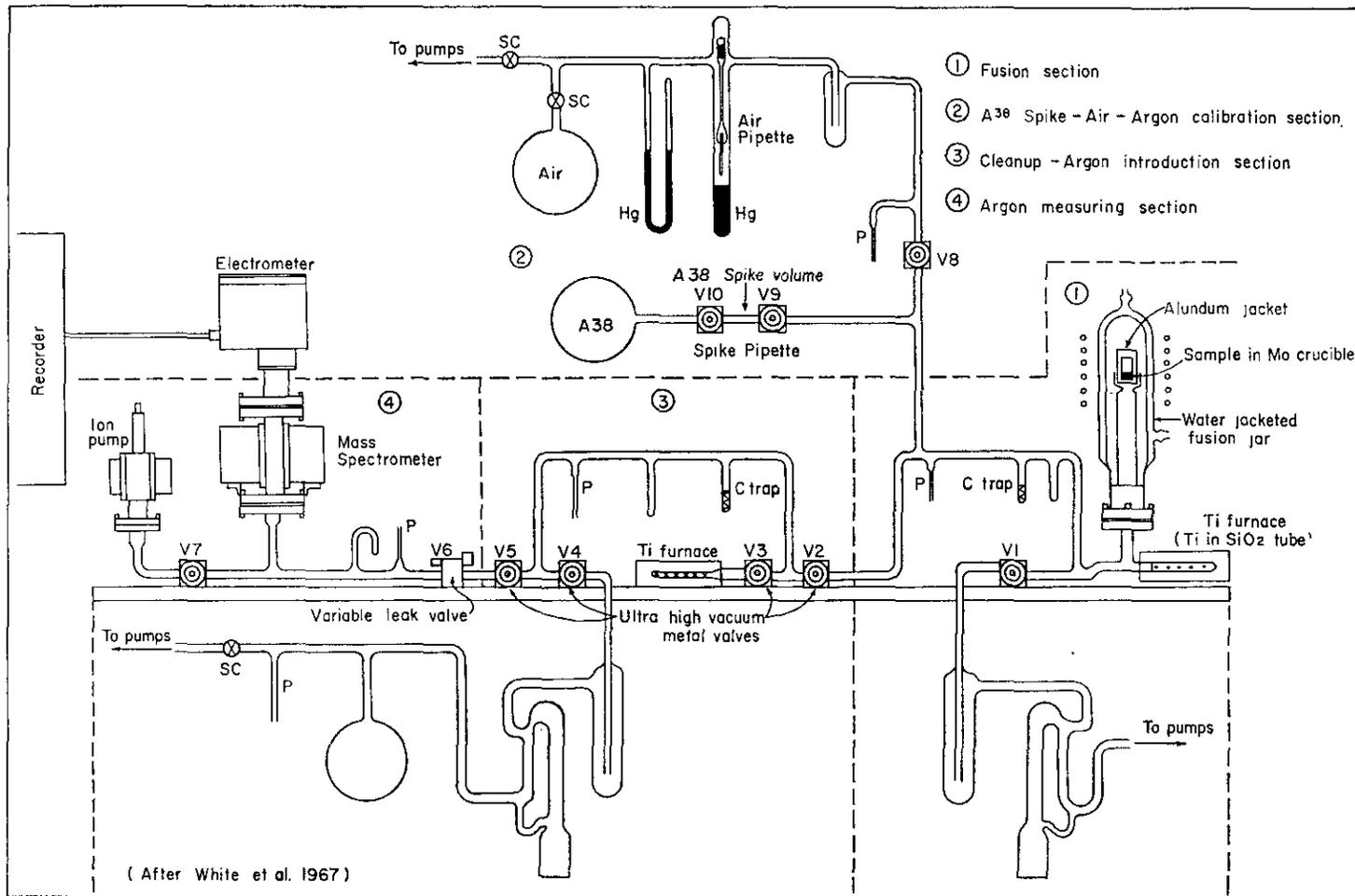
Fig. 13. University of British Columbia K/A laboratory and analytical system.
