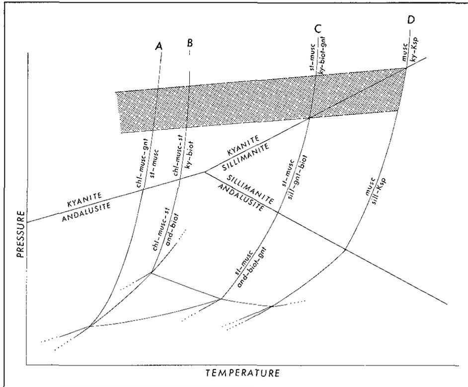
Figure 8. Petrogenetic grid showing limits of temperature and pressure near the gneiss contact.
