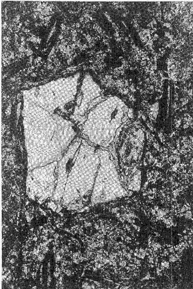
Plate 38. Photomicrograph of an altered pyroxene crystal in a matrix containing abundant altered mica; dike, Bush River area. Long dimension of photograph is 2.5 mm.
