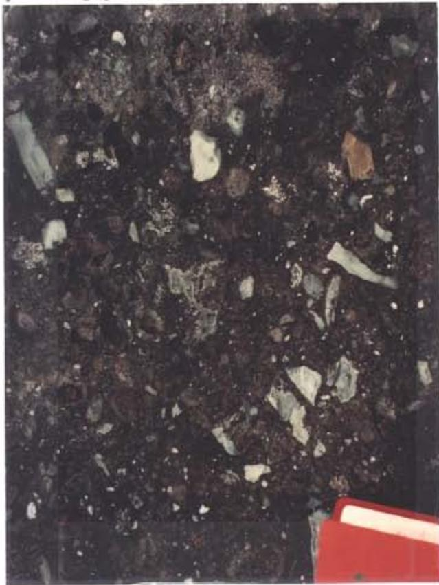
Plate 33. Dark green weathering breccia, Bush River area. Clasts are smaller and less abundant than in rusty mega breccia.
