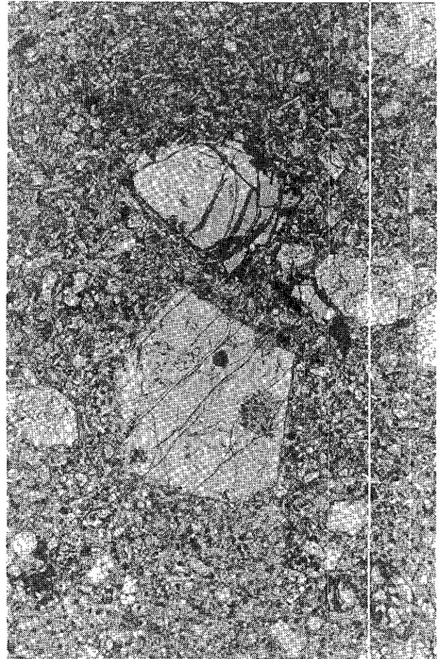
Plate 51. Porphyritic volcanic rock, Russell Peak diatreme. Large euhedral grains are zoned, titaniferous clinopyroxene phenocrysts; the large anhedral crystal is an altered olivine phenocryst; the microphenocryst population consists of titaniferous clinopyroxenes, feldspar laths and opaque oxides. Long dimension of the photo micrograph is 7 mm.
