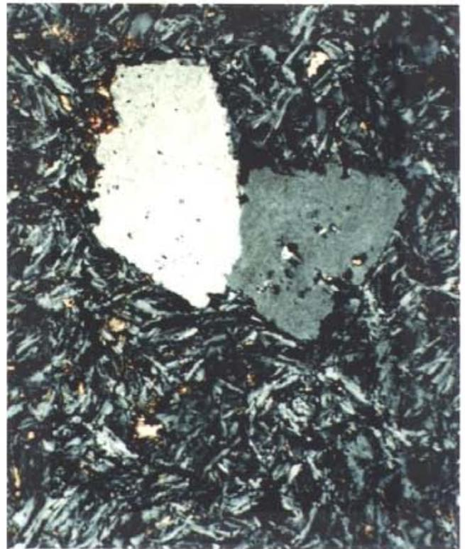
Plate 12. Typical trachyte, Kechika area, note feldspar phenocryst in a matrix predominantly consisting of felted feldspar laths with minor disseminated carbonate and opaques.
