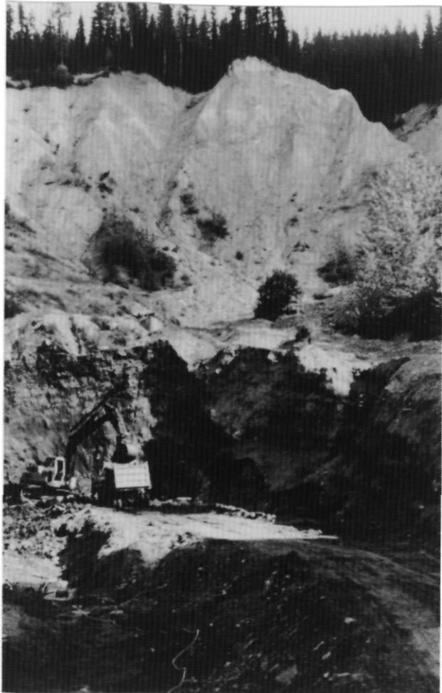
Plate 35. Thick glaciogenic overburden overlying buried paleochannel deposits near Keithley Creek (Location 22). The current operation is mining paleochannel gravels along the bedrock surface at the base of the old channel.
