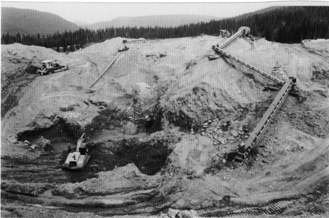
Plate 16. Mining buried paleochannel gravel on a high bench above Devils Lake Creek at the Streicek mine (Location 23).
