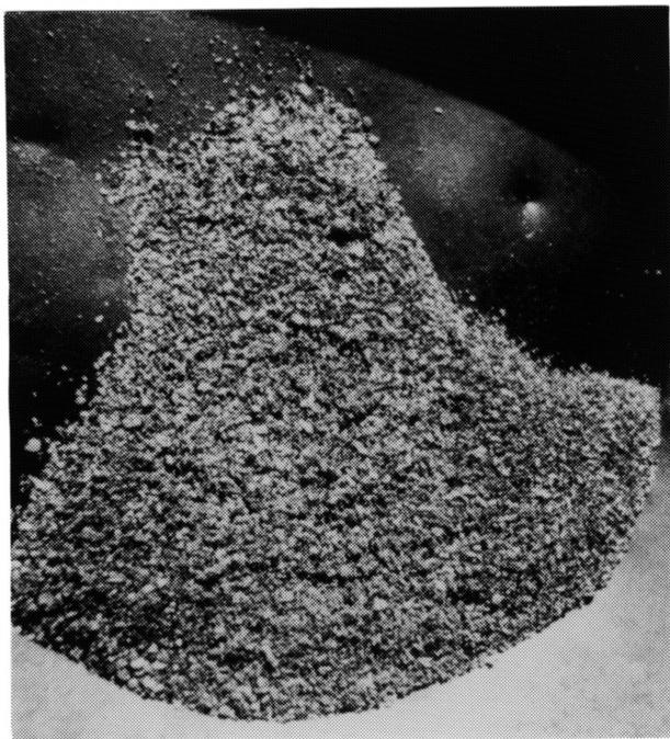
Plate 13. Small, flattened gold particles with rounded edges typical of gold found in braided stream environments.
