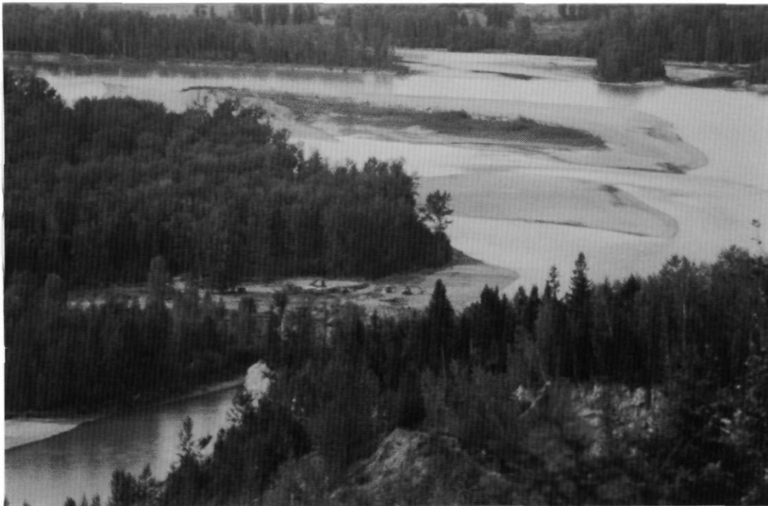
Plate 40. Placer mine recovering fine gold from sand and gravel deposits on a point bar on the east bank of a large meander in the Fraser River north of Quesnel (Location 47) where gold is preferentially deposited during spring floods.
