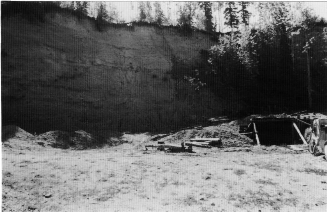
Plate 5. Underground mine in auriferous Miocene gravels north of Horsefly townsite (Location 4). The 25-metre thick overburden sequence consists of horizontally bedded, sandy, small to large-pebble gravels with interbedded, large-pebble to cobble gravels at the base of broad, trough-shaped units. They are interpreted as glaciofluvial gravels deposited in aggrading, braided stream channels. A few metres of glacial diamicton of Late Wisconsinan age caps the exposure.
