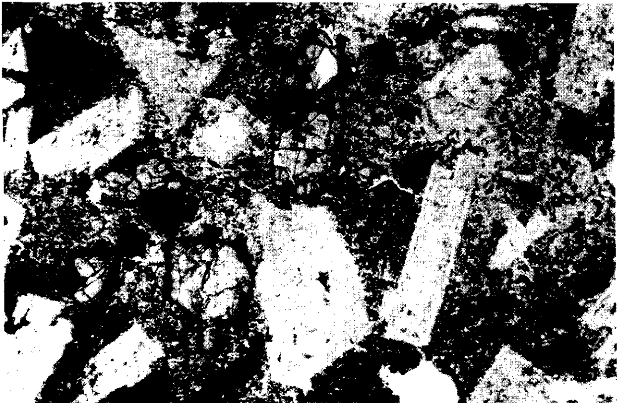
Photo 24. Photomicrograph of crowded diorite porphyry in Chuchi Lake succession. Clast in agglomerate. Unlike the porphyries at Mt. Milligan and BP-Chuchi, there is no potassium feldspar in this rock. Note large apatites with brown rims. Field of view (short dimension) 3 millimetres.
