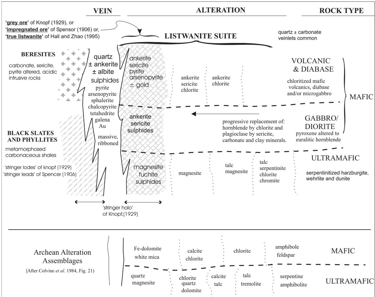
Figure A.2. Schematic representation of alteration products for different ophiolitic host rocks marginal to gold sulphide bearing quartz veins
