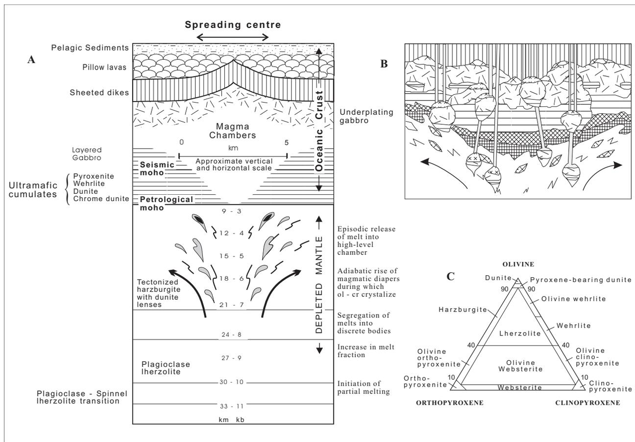
Figure A.1. Idealized oceanic crustal section illustrating the rock types and their relative position of formation within an idealized oceanic spreading centre, modified after Gass (1980), B. Multiple intrusive character of oceanic spreading centers after Ash (1990), C. Classification and nomenclature of ultramafic rocks in the olivine-orthopyroxene-clinopyroxene prism after Streckeisen (1975).
