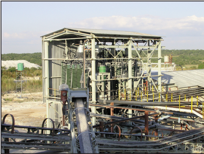
Figure 8. Original (circa 2004) industrial-scale processing plant (spiral module 1) at Marropino, Mozambique. The Marropino pegmatite, which was at one time considered as the second largest Ta producing deposit is also well known for gem-quality morganite (pink beryl).
