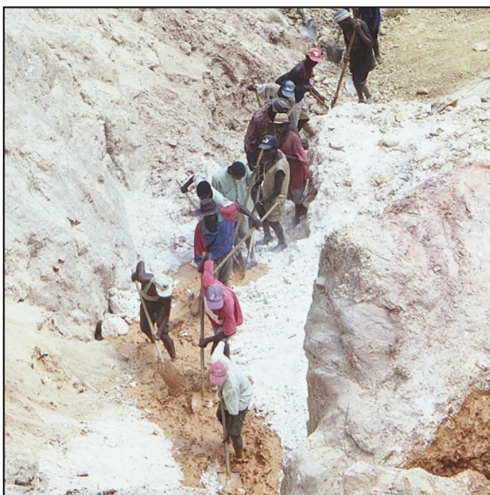
Figure 10. Ground sluicing at Nyabitare beryl–Sn–Ta–Nb-bearing weathered pegmatite, producing high grade tantalum–tin concentrate (western Rwanda). Ground sluicing is a simple technique of primary concentration, favoured by artisanal miners, as no power is required.
