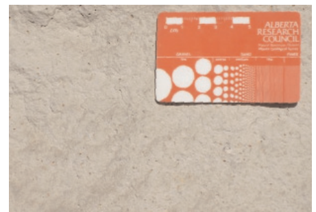
Figure 8. Detail photograph of Haddington Island Andesite.
