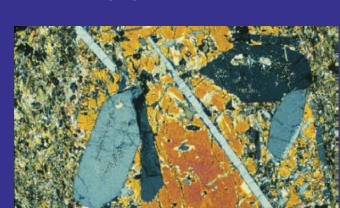
Dyke phase with orange salite pyroxene, grey euhedral apatite inclusions. XPL, FOV = 2.8mm
