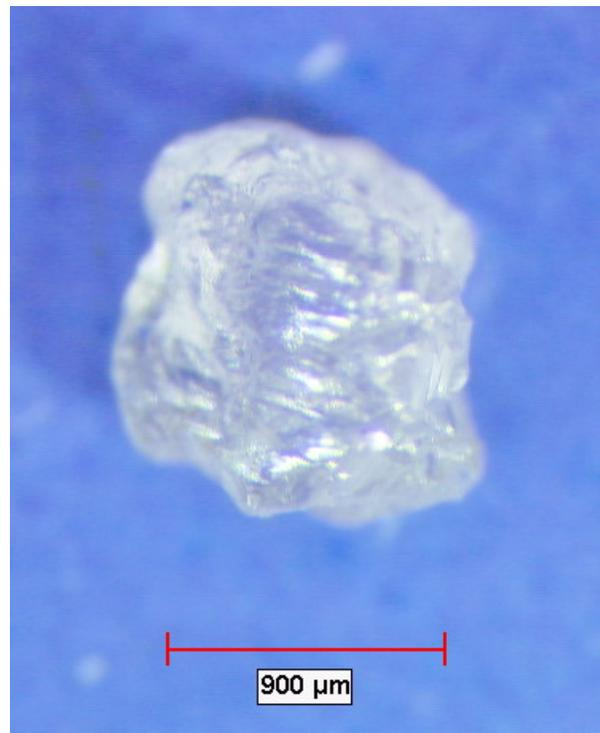
Plates 1a and 1b: Colourless diamond identified in the heavy mineral concentrate of the sample NEBC-11. There is a distinct possibility that this diamond was derived from samples processed prior to sample NEBC-11 or may have come from samples belonging to a previous client (contamination). See sections "Diamond and Fluorite" and "Discussion & Recommendations" for possible implications of this find on diamond exploration in Northeastern British Columbia.
