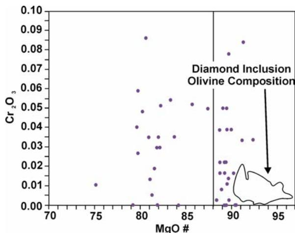
Figure 11. Olivine Cr<sub>2</sub>O<sub>3</sub> - Mg# discrimination plot. Olivines with the Mg# greater than 88 are commonly, but not uniquely, associated with kimberlites. Twenty six grains from this study have Mg# greater than 88. The outline of olivine compositions found as solid inclusions in diamonds is from Fipke *et al.* (1995). None of the grains recovered during the current study from this study fit that profile.
