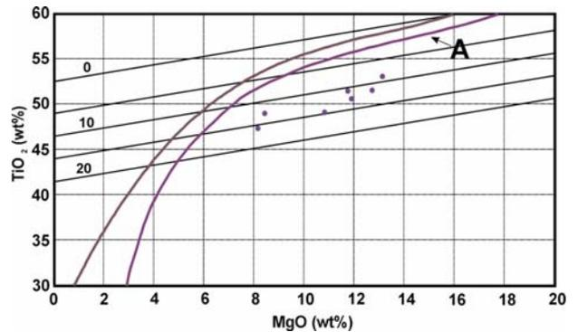
Figure 9. Ilmenite  $\text{TiO}_2$  - MgO discrimination plot (after Wyatt *et al.*, 2004). Seven grains plot within the kimberlite field, which is located to the right of the curve marked 'A'.
