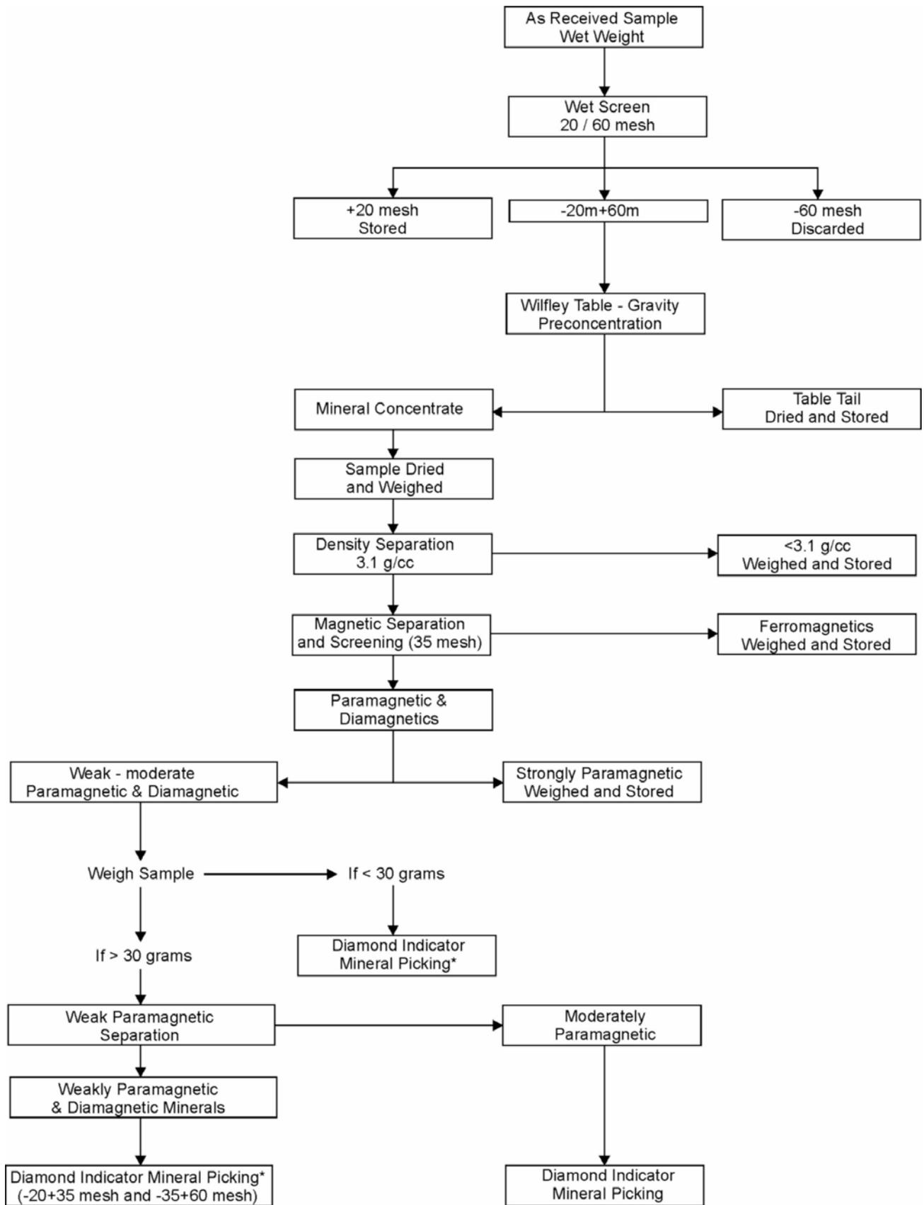
Figure 3. Diamond indicator mineral extraction flow sheet. \* indicates primary diamond indicator mineral fraction. Source: SGS Lakefield Research Limited.
