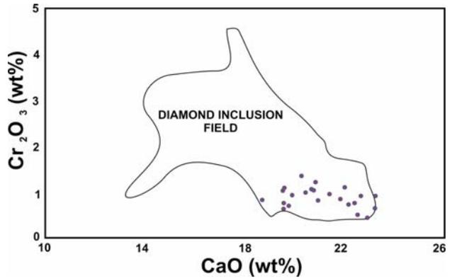
Figure 6. Clinopyroxene;  $\text{Cr}_2\text{O}_3$  - CaO plot. The outlined field represents the composition of clinopyroxenes found as inclusions in diamonds (Fipke *et al.*, 1998)
