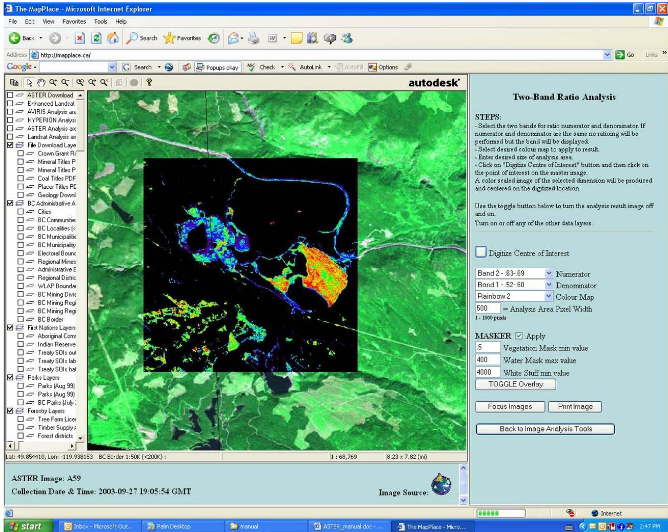
Figure 11. Application of the Two-Band Analysis ( $A2/A1$ ) with Masker to the ASTER overlay illustrated in Figures 7 through 10, over Brenda Mine. This ratio is used to identify possible iron oxides in the image. This has brought the focus of this analysis to the area of the tailings and dam which have the highest value from a ratio of the two bands in the area.
